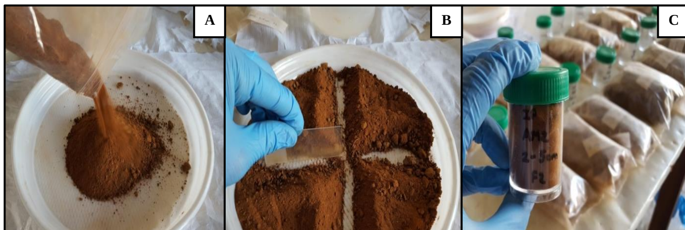
Figure 2.7. Bulk/cone and quarter method for soil homogenization. Sample was poured in a cone shape (A). Plastic plate and glass slide (B) were cleaned between samples whereas a new plastic knife was used for each soil sample. Samples were stored in sealed plastic specimen bottle for processing (C).
