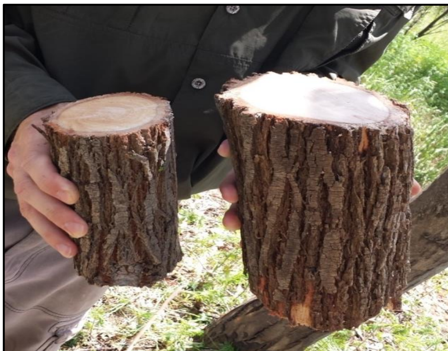
Figure 2.6. Wood sections were collected for density and volume measurements. Wood section (on left) was cut at 1.1 – 1.3 magl ground (to preserve circumference where DBH was measured for allometric equations) whereas the wood section (on right) was cut at 0.2 – 0.4 m (to preserve circumference where SBC was measured at 0.3 magl).
