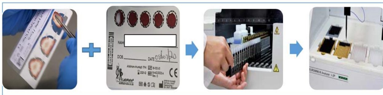
Figure 23: The processing of PSC and DBS using the automated EUROIMMUN analyser I-2P instrument.
