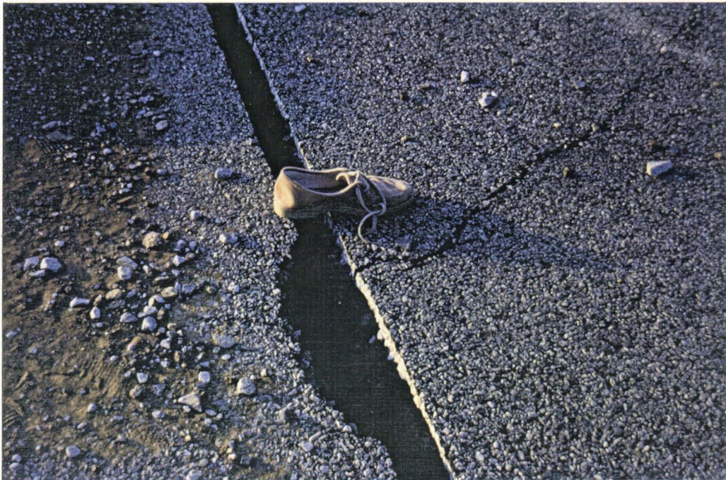
PLATE 8 The same slot after mining, indicating the amount of closure.
