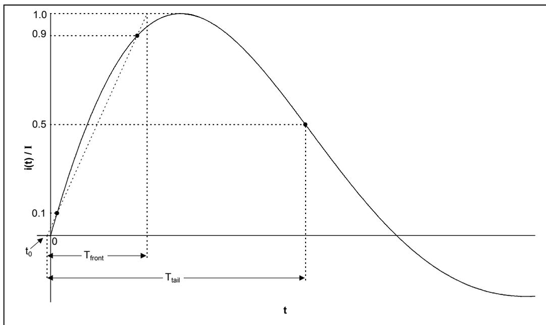
**Figure 2.1:** Current impulse definition as per IEC 60-1:1989
