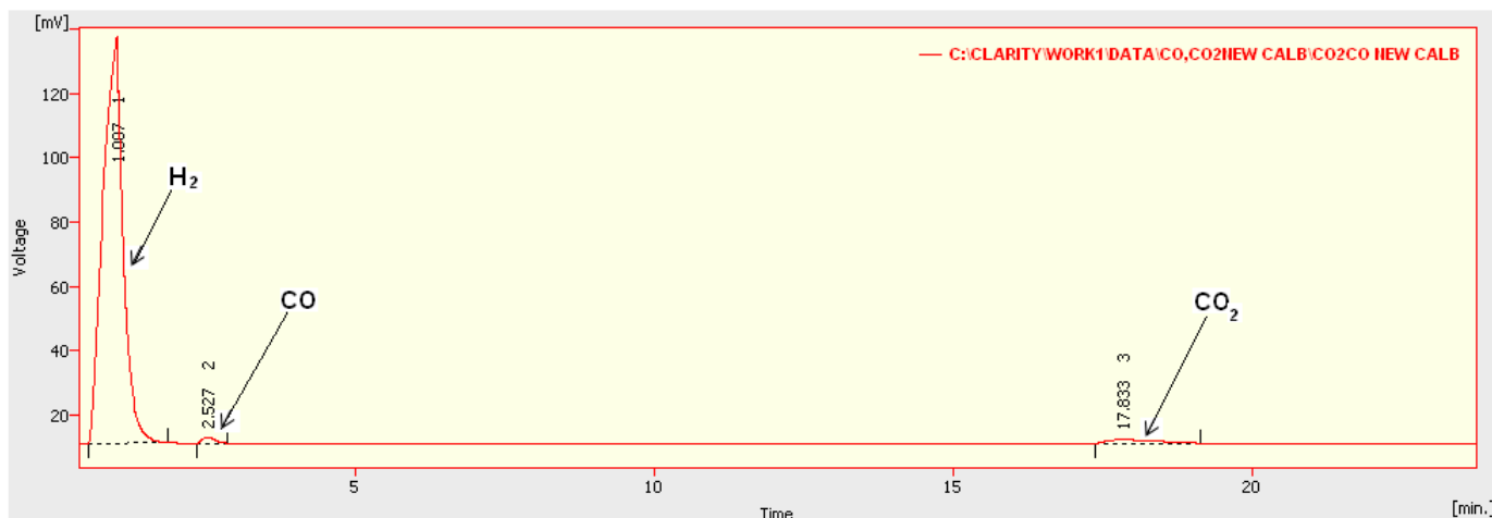
Figure 3.12: Blank run for the selective methanation of CO in a CO_2 and H_2 gas mixture.
