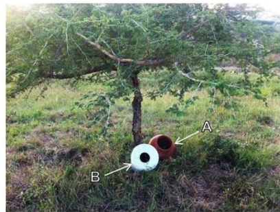
Figure 2. Ceramic pot (A) and modified plastic bucket (B) used for adult Anopheles mosquito surveillance, Mpumalanga and KwaZulu-Natal Provinces, South Africa.
