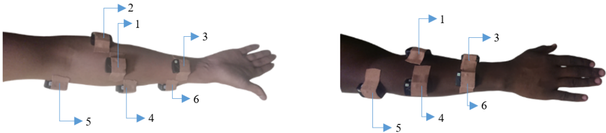
Figure 3.7: Forearm placement of sEMG sensors directly above target muscles.
