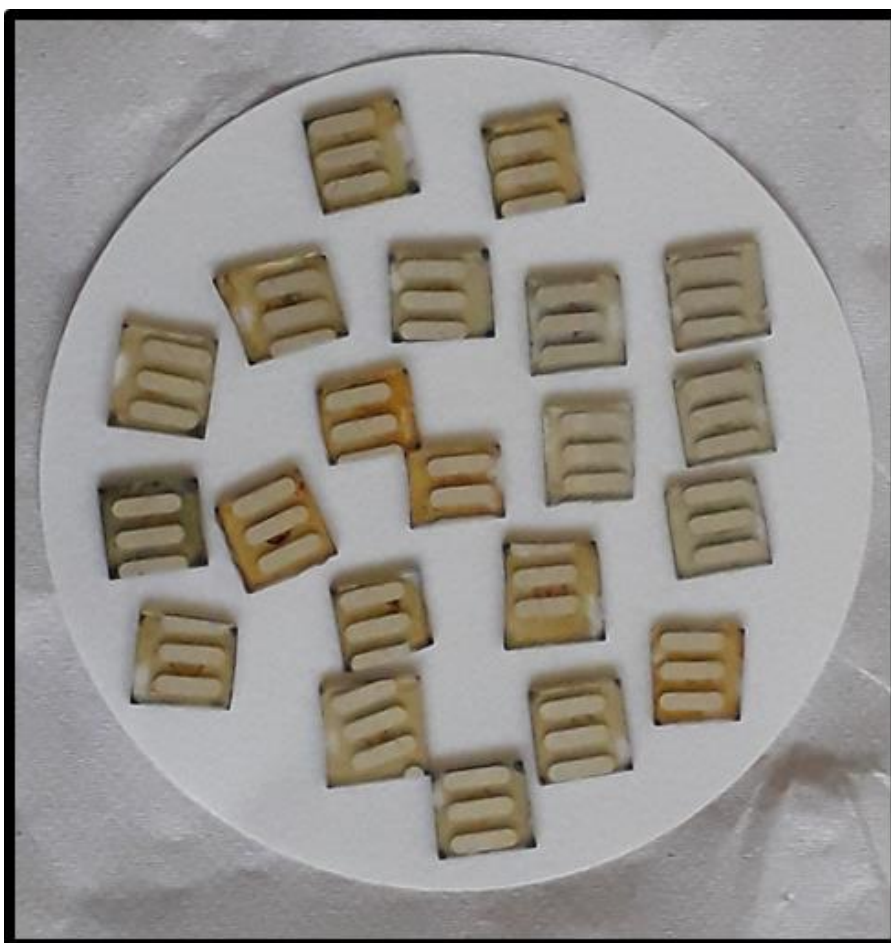
Figure S1: Different fabricated organic bulk-heterojunction devices.
