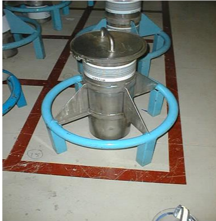
Figure 2.7: A container designed to keep a safe distance from another container [source: photo obtained from a colleague who visited Springfields Fuel Ltd.].
