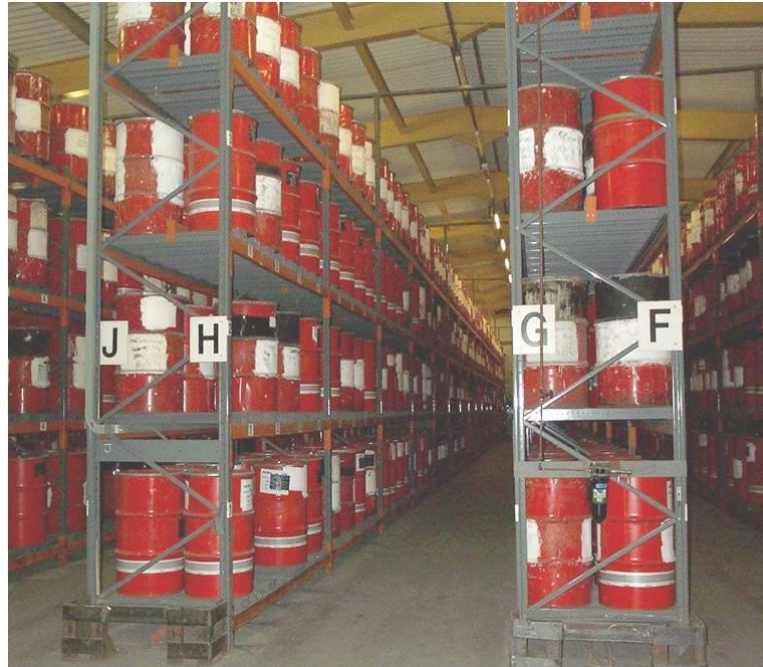
Figure 2.8: A moderation safe storage area for canisters containing fissile material [Source: photo obtained from a colleague who visited Springfields Fuel Ltd.].
