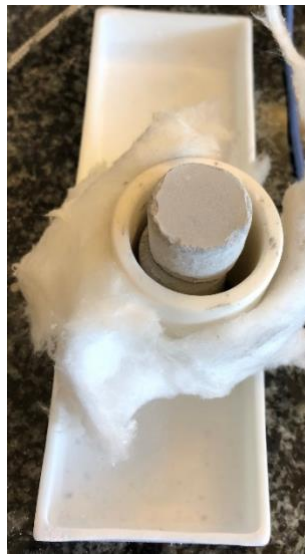
Figure 3.3: Setup of melting crucible with ceramic blanket.
