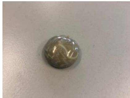
Figure 4.11: Crystallized cast pyrophyllite.
