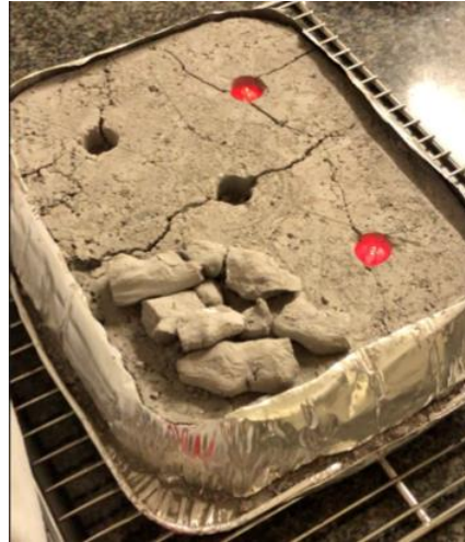
Figure 3.6: Cast samples cooling in pyrophyllite bed.
