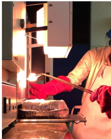
Figure 3.5: Casting of melted pyrophyllite.
