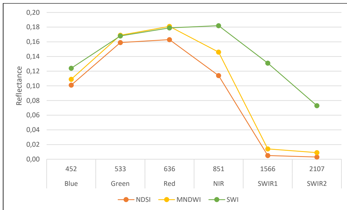
Figure 16: Surface water spectral reflectance extracted from NDSI, MNDWI and SWI using Landsat 9 OLI.
