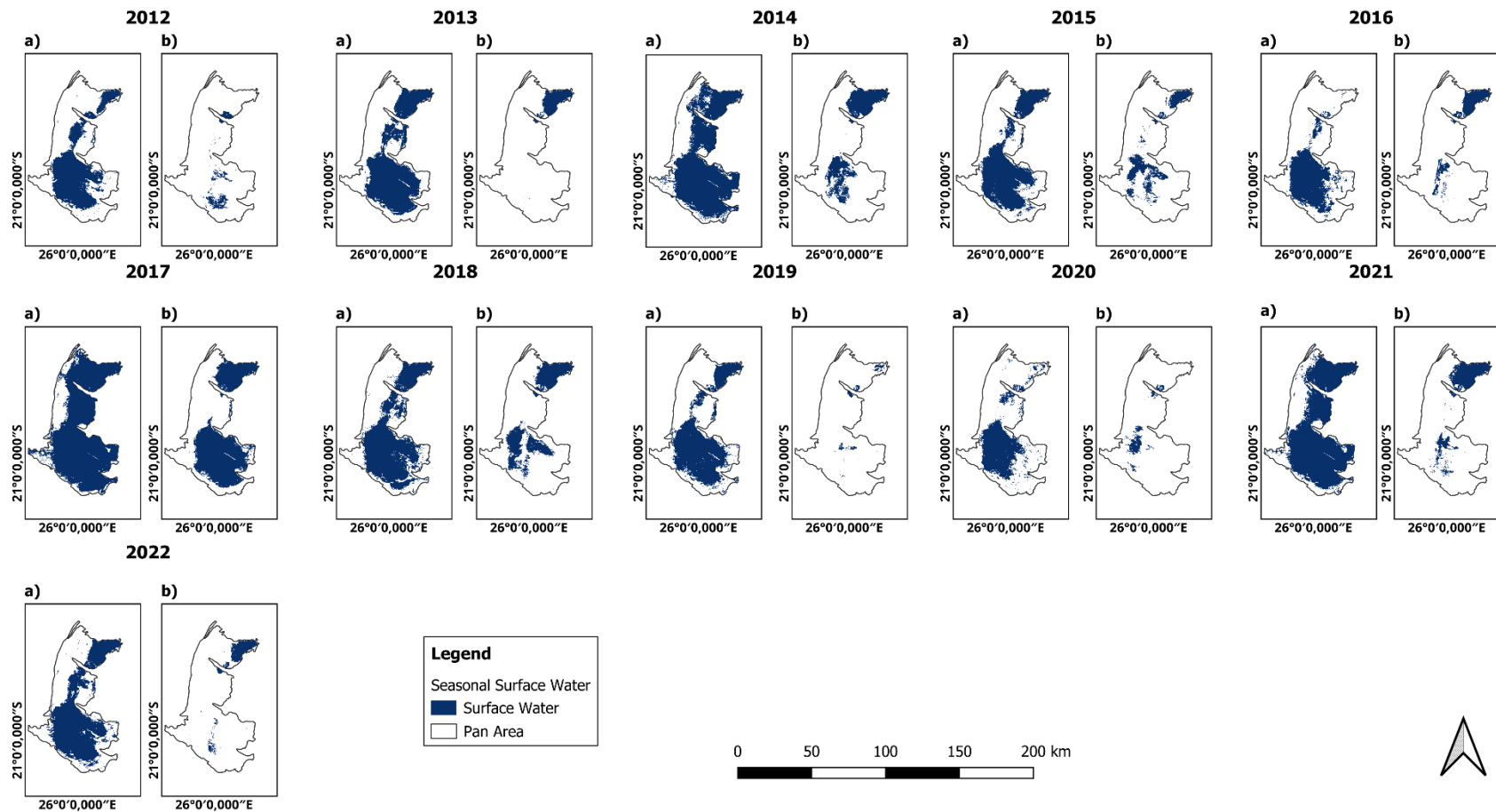
Figure 18: Spatiotemporal maps of surface water area using SWI during the a) wet season (January to March) and b) dry season (August to October) from 1992 to 2022.
