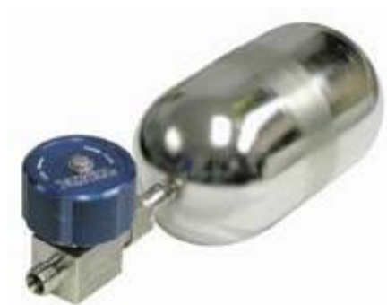
Figure 3.10 Canister for sampling leaf air
