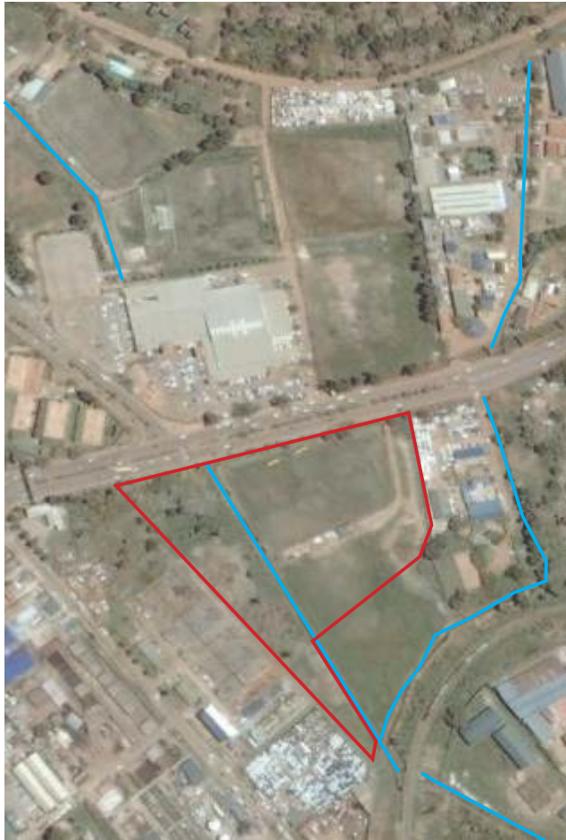
Figure 4.17: Lugogo junction in 2008; With the development of Lugogo Shopping mall, the porous surface of what used to be a big part of the one the sports fields was not the replaced by hard impermeable paving of the parking which would not encourage drainage.
