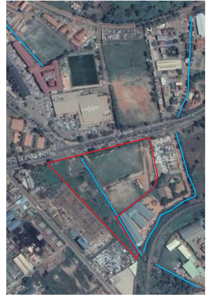
Figure 4.22: Lugogo junction in 2019; Due to the development over the years, the site floods after heavy rains during the rainy season because most of the flood plains were encroached upon.
