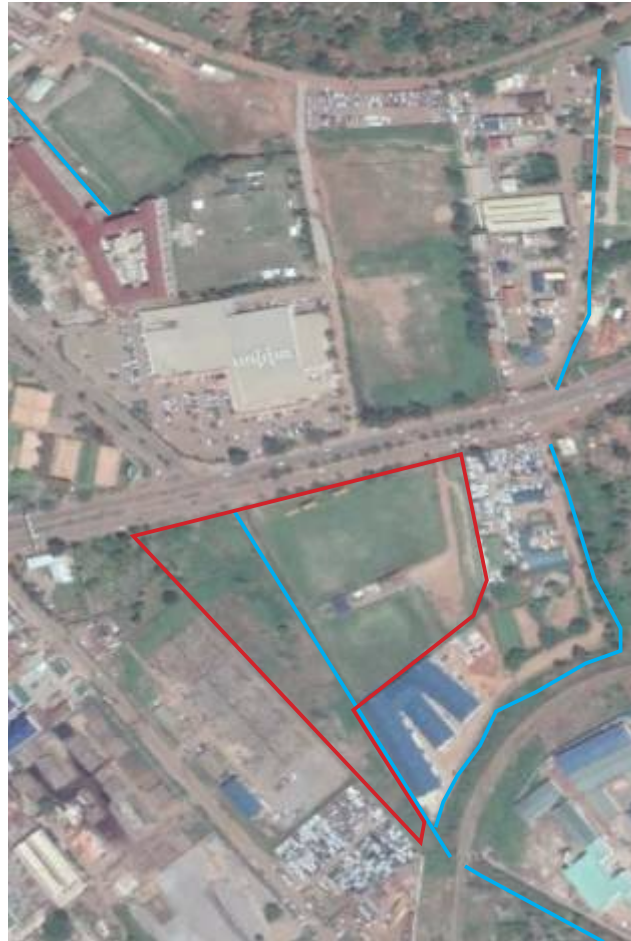
Figure 4.18: Lugogo junction in 2010; The development of another shopping mall, forest mall, and North of Lugogo Shopping mall also encroached on the green space which was in close vicinity to an open drainage channel as was the case with Lugogo Shopping mall. The development of the factory south of the site interfered with the flow of water towards the drainage channel. This also reduced the size of the flood plains.
