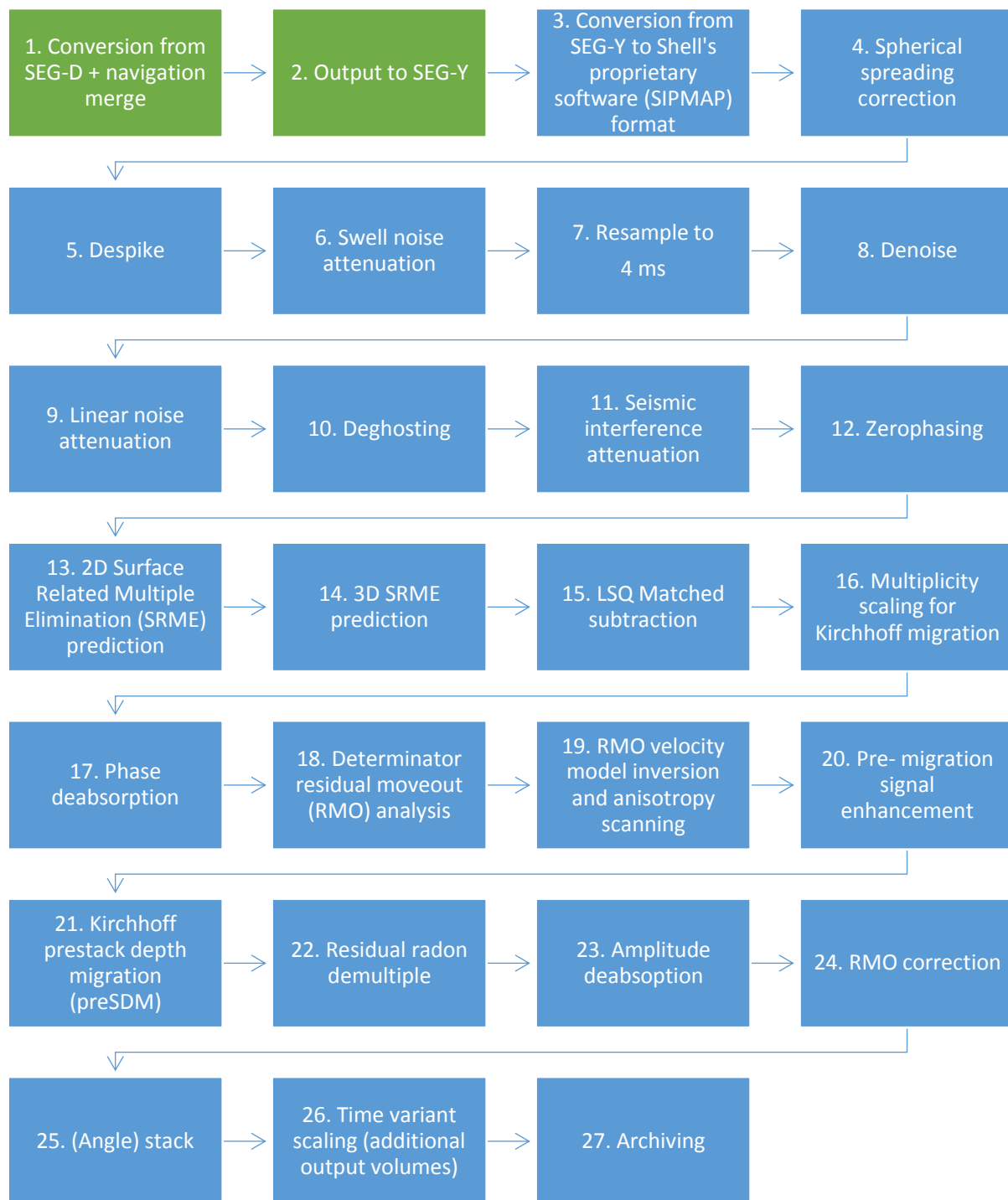
Figure 3.2. Processing flow used to process the Orange Basin 3D seismic data. The green box shows processing done by Dolphin Geophysical Polar Duchess. The blue boxes show processing done using SIPMAP (Kramer and Heck, 2014).
