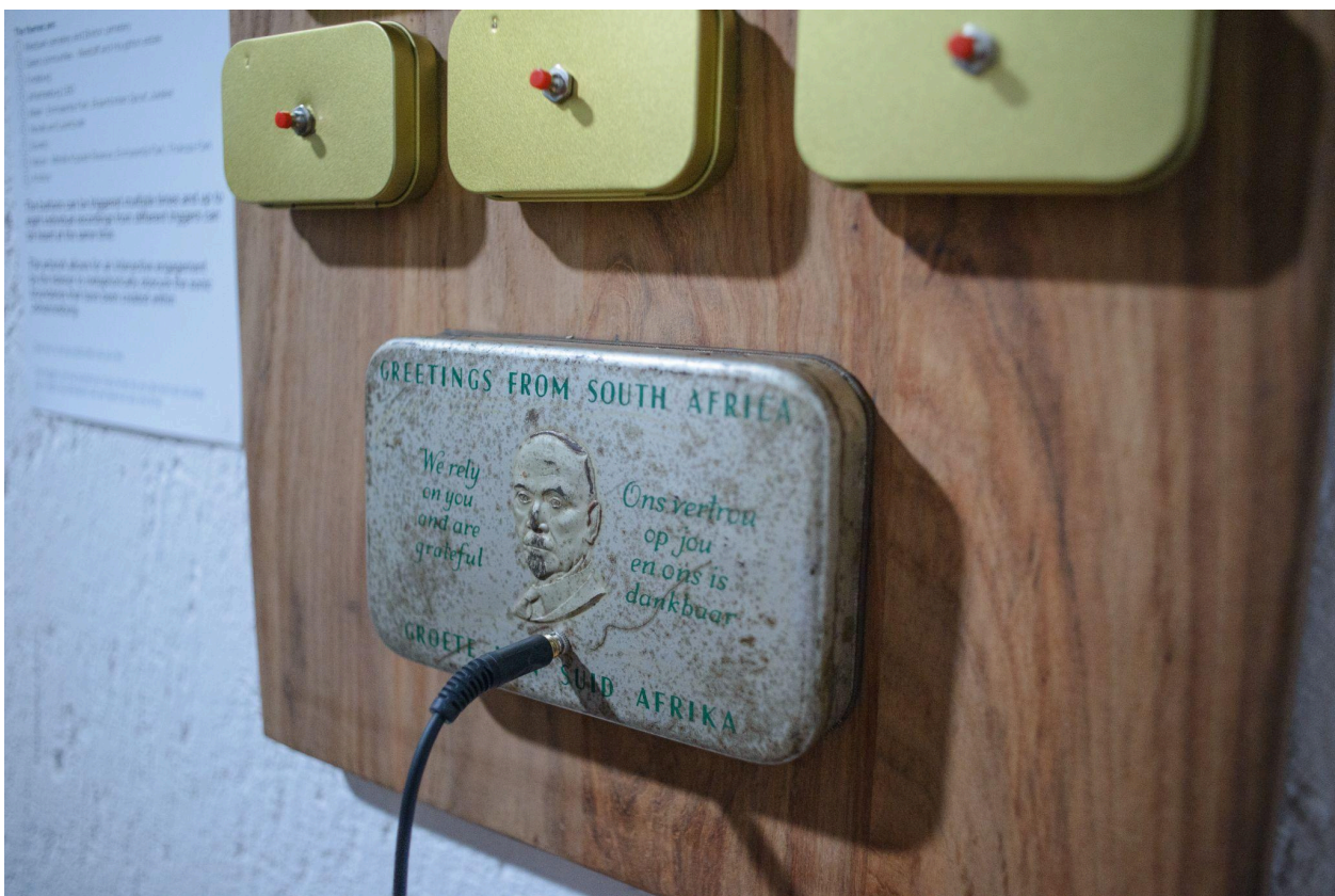
Figure 8.4 The tin box housing the WAV Trigger audio playback device (Haggis, 2025).
