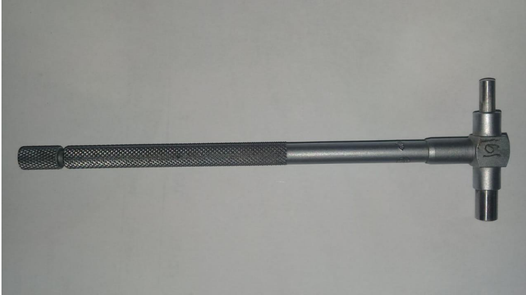
Fig. 3.17 Telescopic gauge used to measure the final height of the specimens, H_f .
