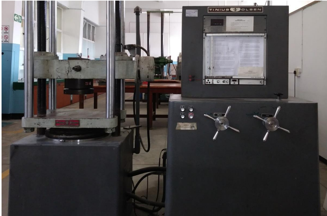
Fig. 3.7 Discrete loading compression machine.
