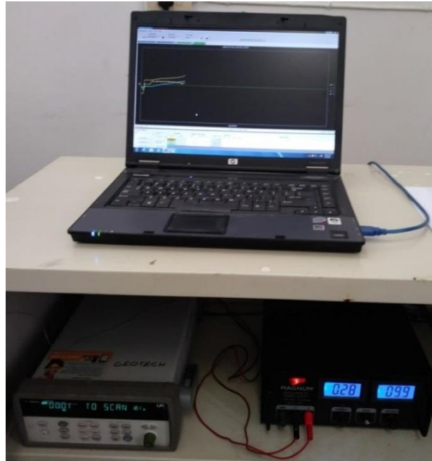
Fig. 3.2 1-D confined compression testing equipment data acquisition system.
