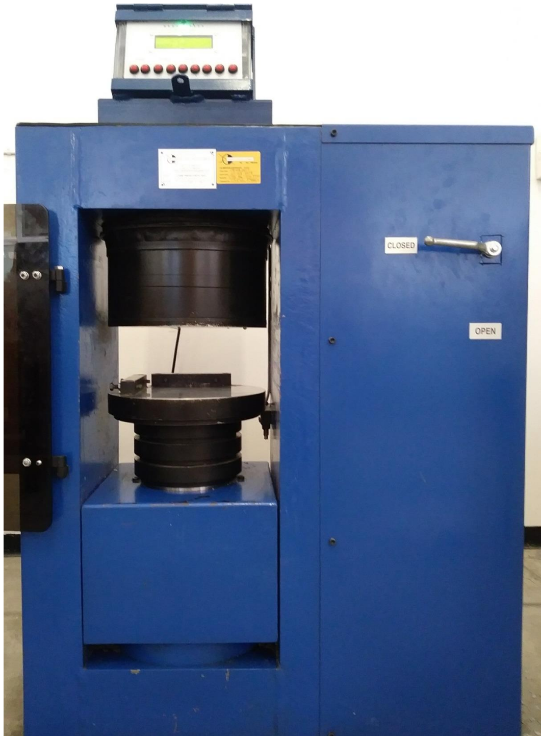
Fig. 3.6 Continuous rate of stress loading compression machine.
