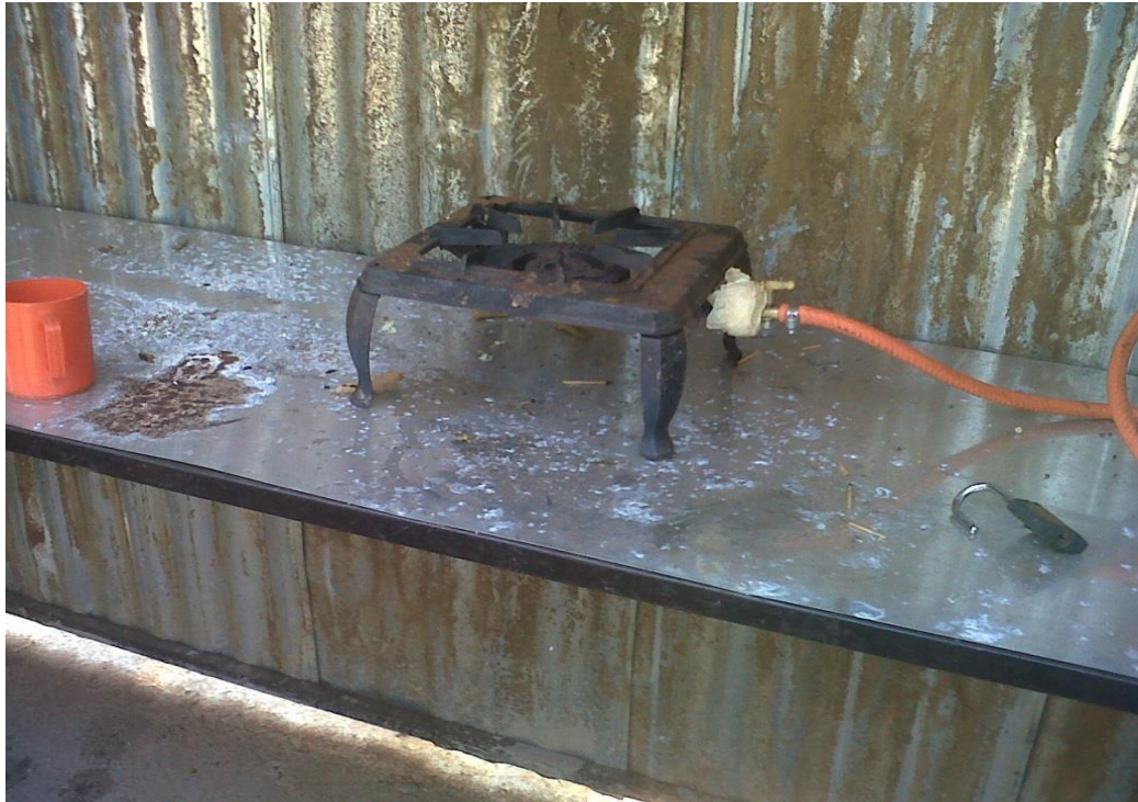
Picture 8: Ready-to-use biogas demonstration stove
