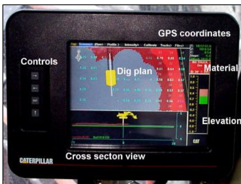
Figure 2.6. Example of loader operator in-cab display (Richards, 2001)
