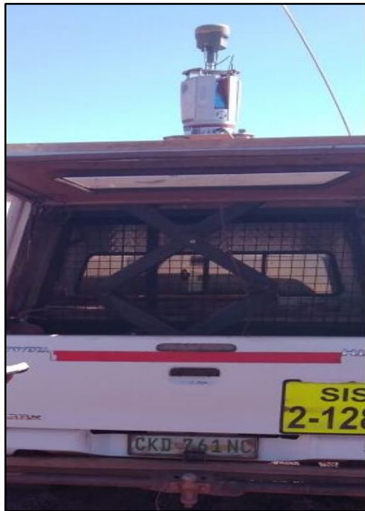
Figure 4.6. Laser scanner mounted on an LDV
