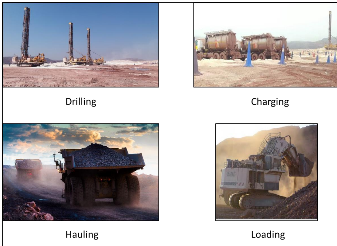
Figure 5.9. Major open-pit mining activities performed at Kolomela
