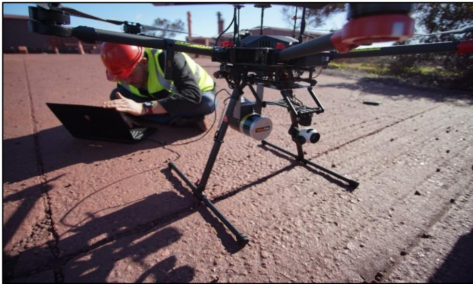
Figure 4.7. RPAS fitted with LiDAR unit
