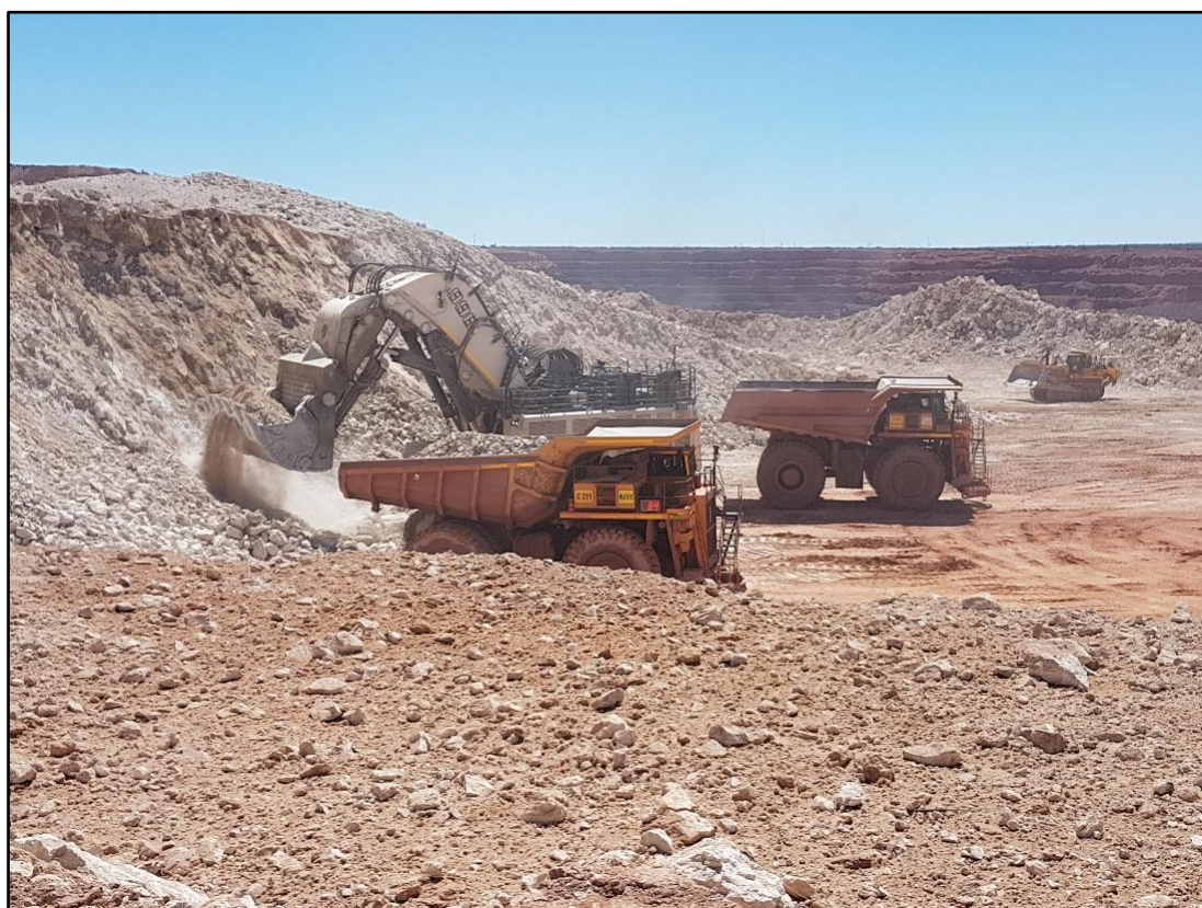
Figure 5.10. Loading of Komatsu 730 trucks with a Liebherr R996 shovel
