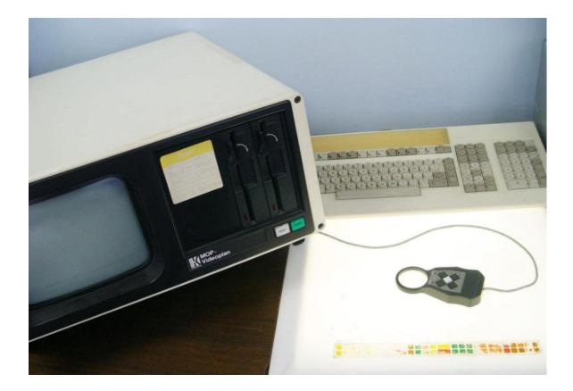
Figure 3.2.1.1 The Kontron Videoplan Digitizing System.
