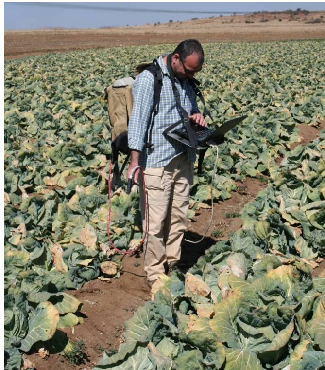
Plate 10 Example of the acquisition of ground spectra using a hand-held field ASD from targets encompassing light to dark materials
