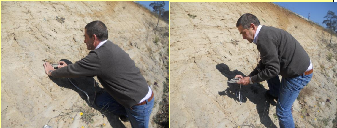
Figure 3-29 Pictures illustrating measurement of dip direction with a compass
