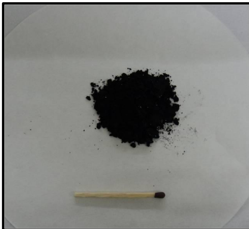
Figure 3.3 Photograph of soot collected from the cyclones (match stick used as reference to give a sense of size).
