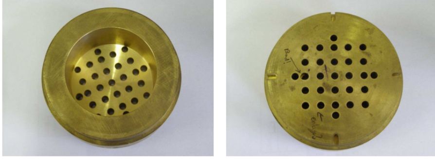
Figure 4.7: Photo of the pepperpot collimator used during experiments. The holes each span 0.41^\circ and the centroids are 0.81^\circ degrees apart.
