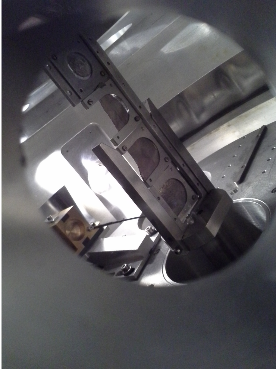
Figure 3.9: A photo showing the target frame used in the PR210 experiment. The lower dispersion sides of the frame has been removed to reduce the amount of scattering from it [54].
