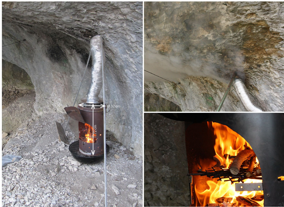
Fig. 2 Experimental device comprising a furnace to introduce the fuel (72×32 cm), a flexible and modifiable chimney, and a basin to avoid anthracological pollution and the rubefaction of the shelter floor. The device blackens a limited area of the wall (formation of black spots)
