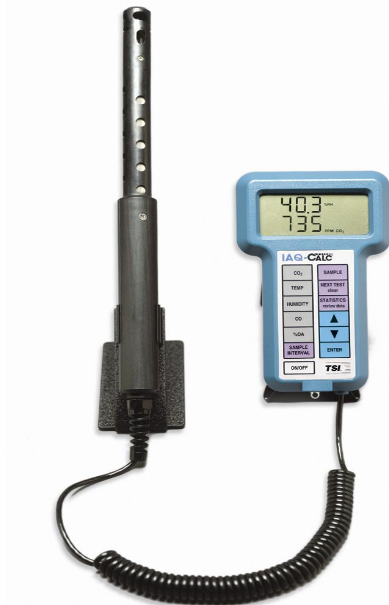
Figure 1: Illustrates the IAQ – Cal. meter model 8760/8762 used for measurement of Environmental IAQ conditions
