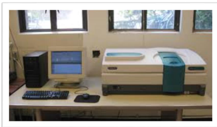
Figure 3.9. A photograph of the Praying Mantis Cary 500 UV-DRS that was used in these studies.
