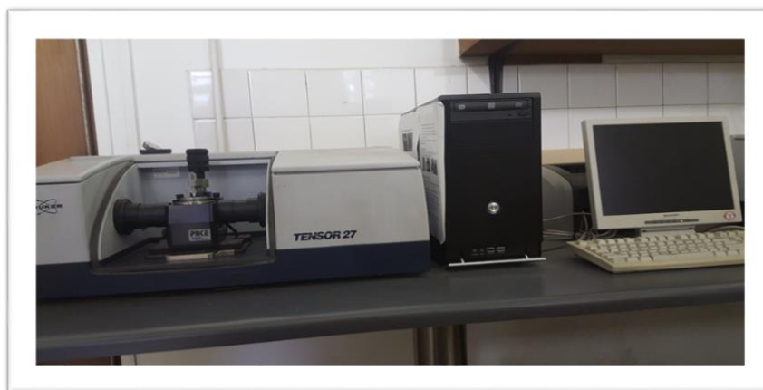
Figure 3.5. A photograph of the Bruker Tensor 27 FTIR spectrometer that was used in these studies.
