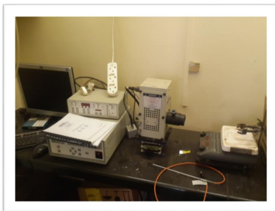
Figure 3.10. A photograph of the Newport model 69911 solar simulator that was used in these studies.
