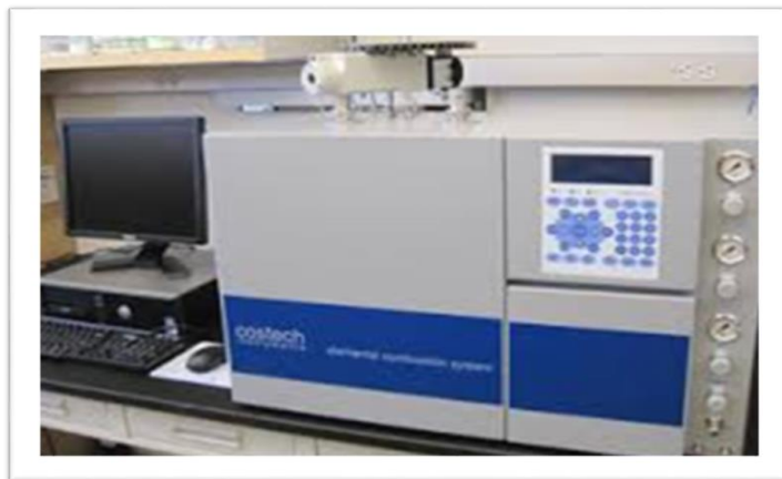
Figure 3.8. A photograph of a Carlo Erba EA 1108 Organic Elemental Analyzer like the one that was used in these studies.
