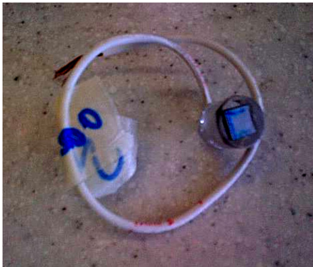
Figure 3.2 Mounting of sample for potentiodynamic polarisation measurements
