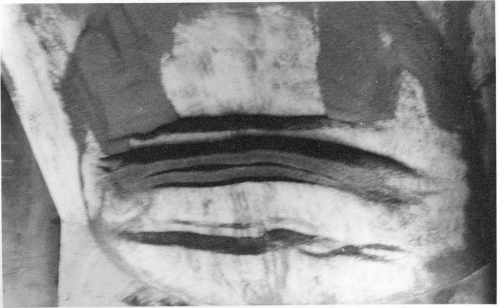
Figure 6.10(c) Secondary failure developing in unfailed wedge pushed out before main failure.
