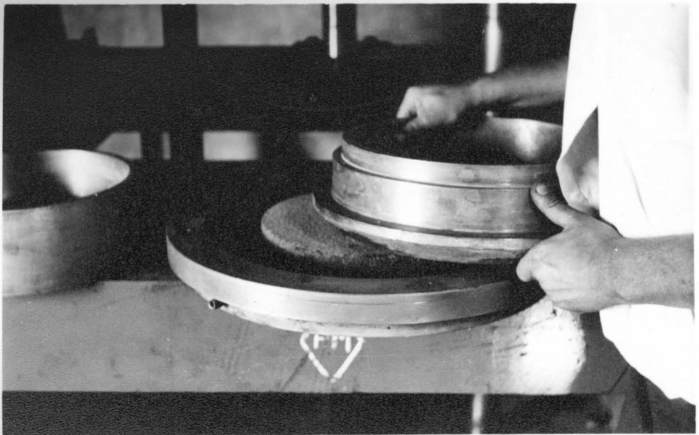
Bottom side plate and bottom drain plate (an Emery wheel with the centre hole filled with lead) placed in position.
