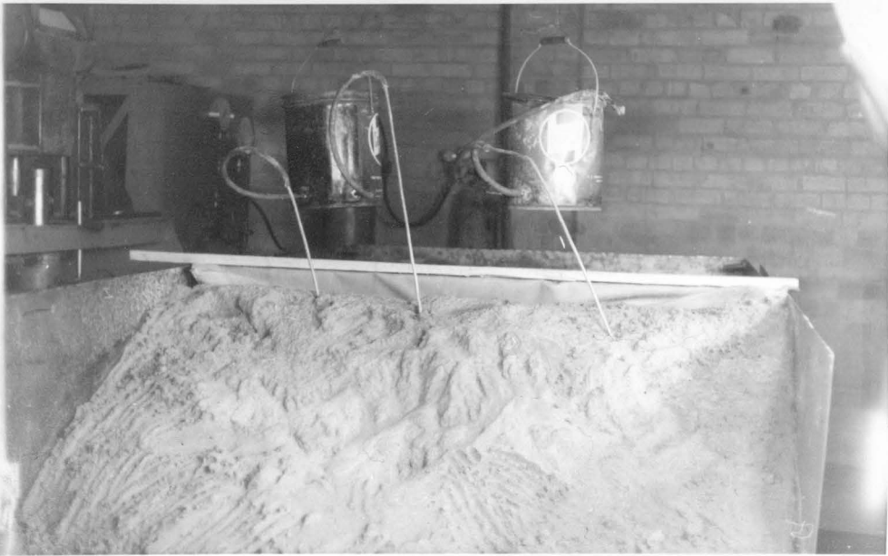
Figure 6.6(d) Failed wedge is covered with a layer of fine and rough sand, and gell pumped into the model. The layer of fine sands contains the gell inside the model.
