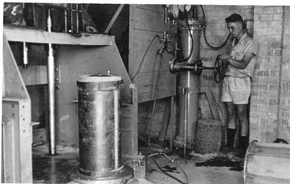
Figure 9.12(h) Top strap tightened, hand pressure control cylinder fitted and negative pressure applied to sample.
