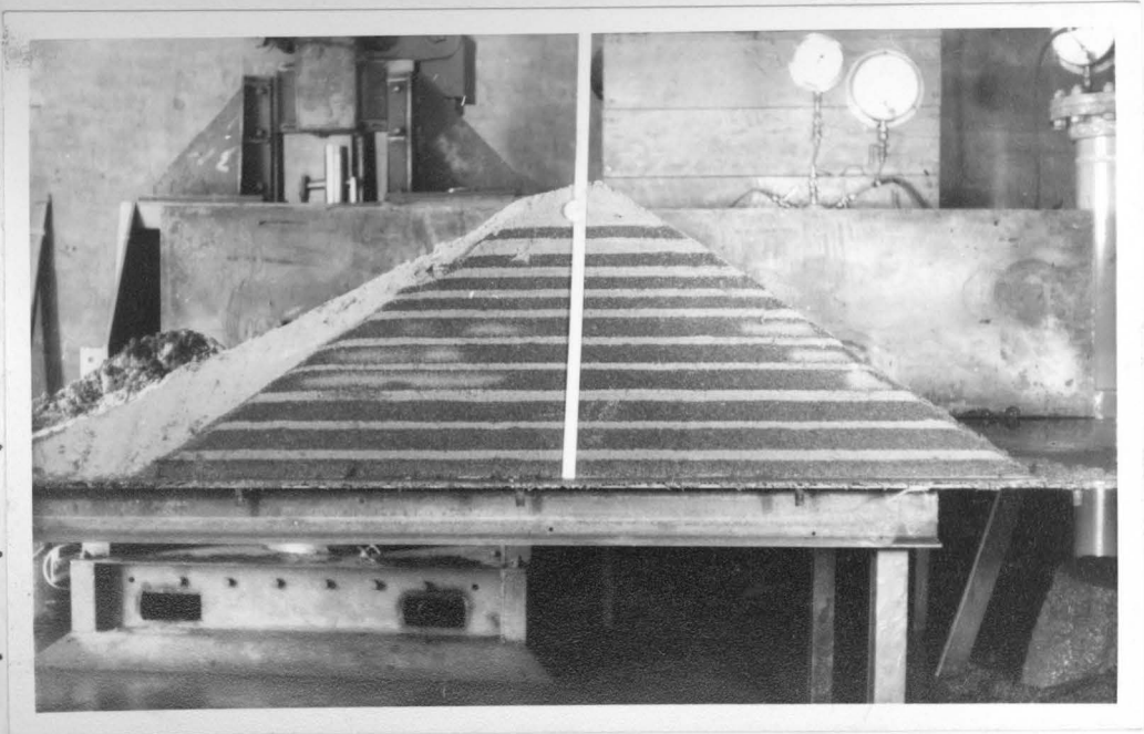
Figure 6.11(a) Cross section of wedge at side plates of the failure.
