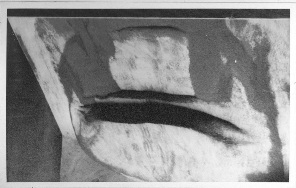
Figure 6.10(b) Main failure developing in model wedge.
