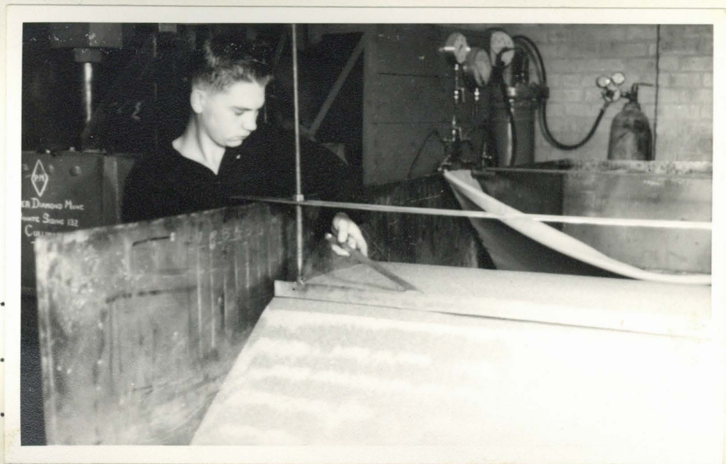
Figure 6.5(e) Photograph shows method employed to form the edges of the layer to the angle of repose. The blade is set at the edge and sand carefully pushed below the blade till the angle is correctly formed.
