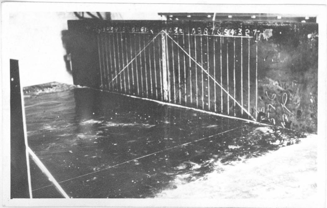
Figure 6.5(a) Model table with tar spread over base and base and side lines chalked.
