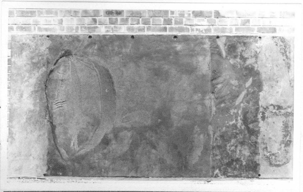
Figure 6.12 Deformation of the tar on base plate due to failure. Note beginnings of a transverse failure in the tertiary failure zone.
