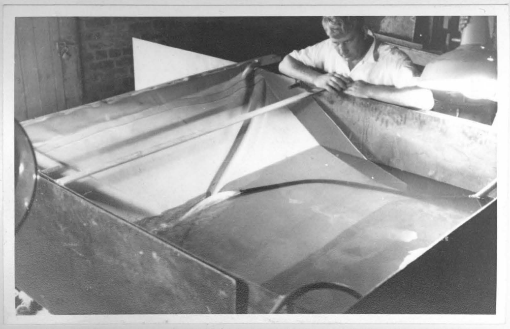
Figure 6.9 Tank being filled to supply water pressure against wedge.
