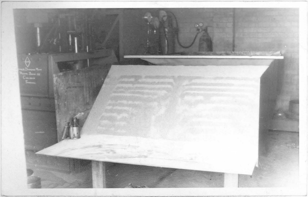
Figure 6.8 Completed wedge with thin rubber membrane of tank in background.
