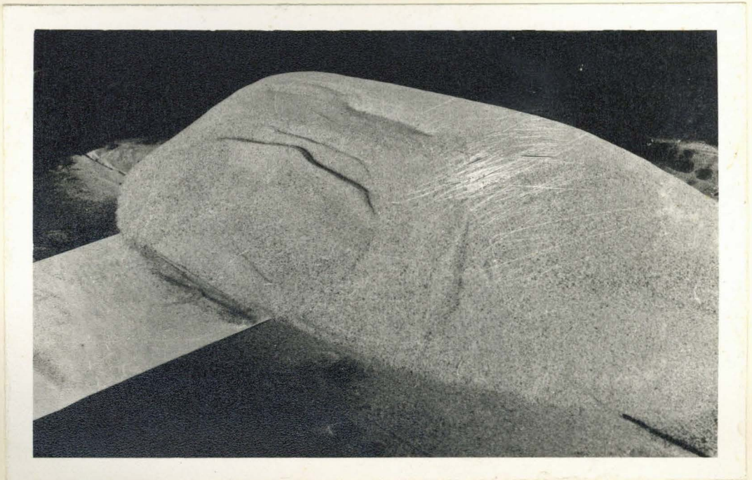
FAILURE OF MODEL BANK FIG 6.1(b)
