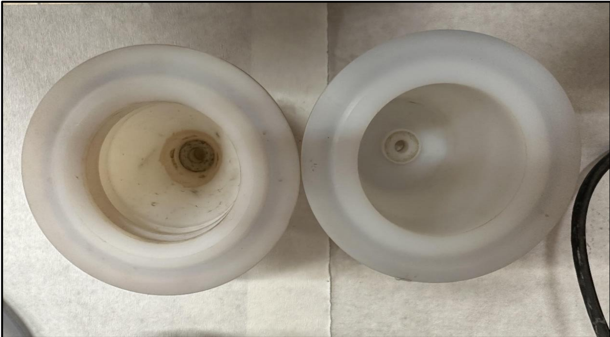
Figure 33: Falcon gravity concentrator bowls showing the fluidized bowl (left) and unfluidized bowl (right)
