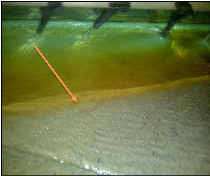
Figure 20: Gold Separation on a Shaking Table (source of photo: Taurean Nair, 2015)
