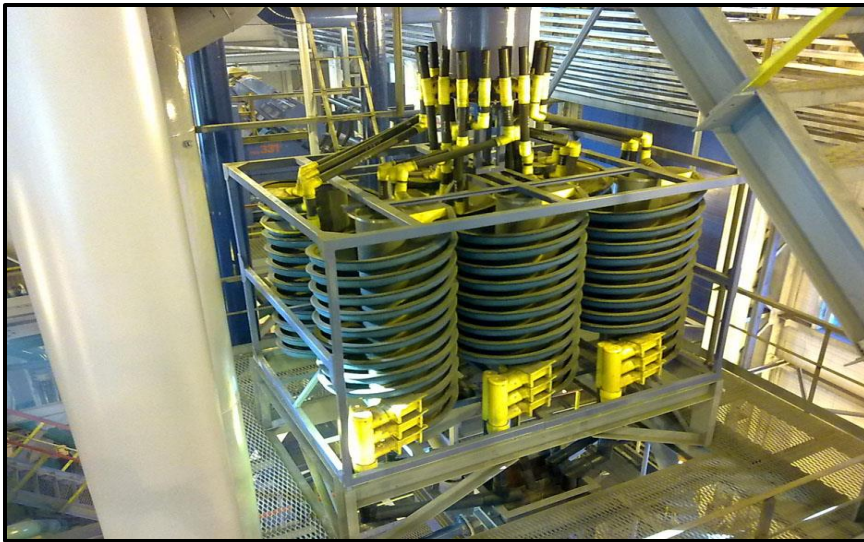
Figure 17: Spiral Concentrator (FLSmith, 2024)
