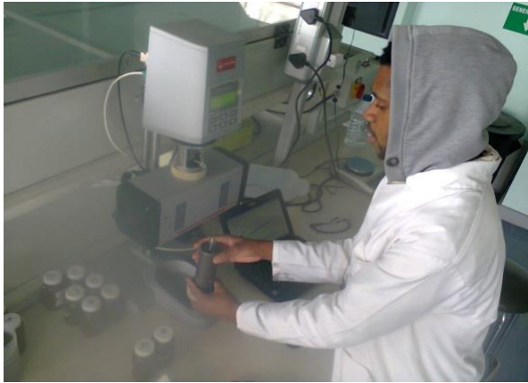
Figure 3.2: RheolabQC viscometer from Anton Paar (South Africa).
