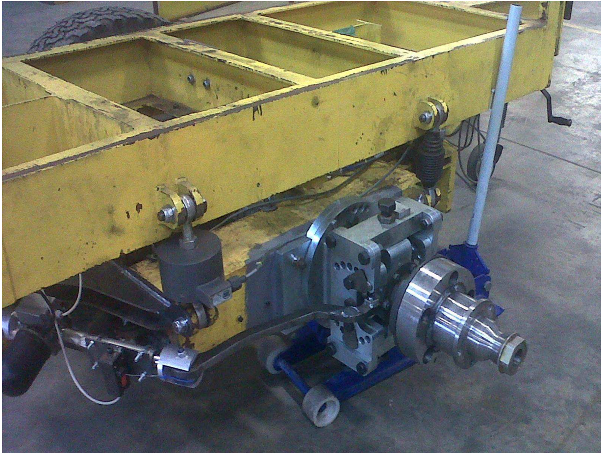
Figure C.2: Hankook Wheel Adapter on the Tyre Tester
