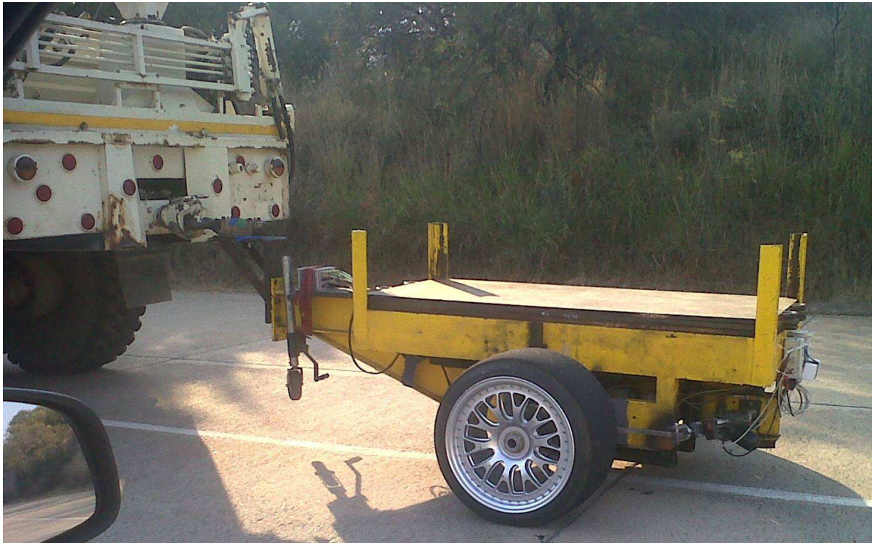
Figure C.7: SAMIL 100 Towing the Tyre Tester
