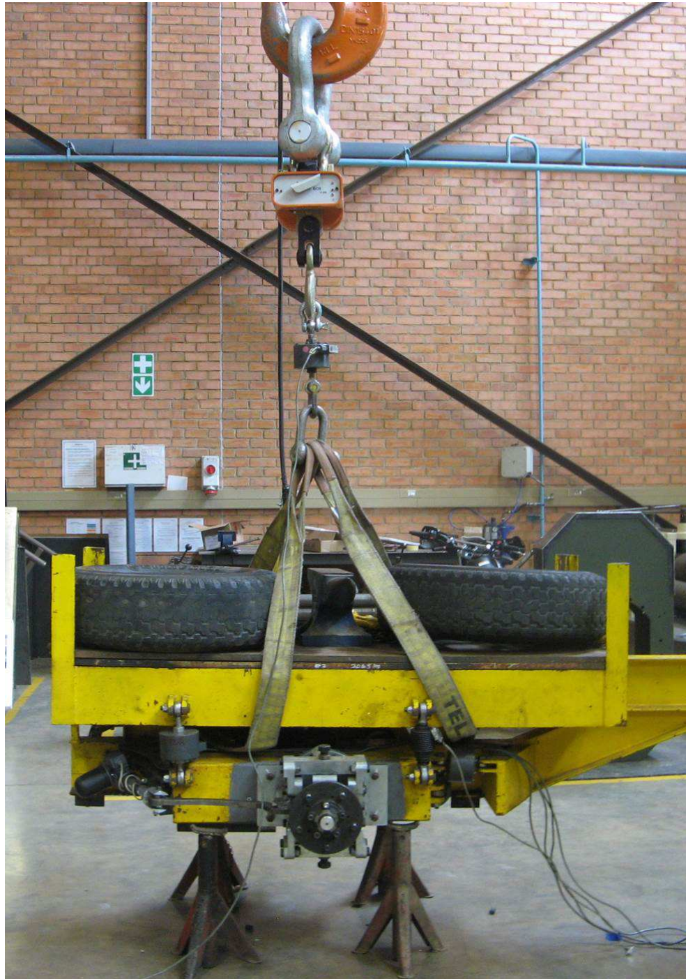
Figure C.3: Calibration of the load cells
