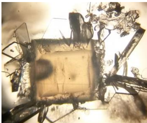
Figure 19: Single crystals of 3,4-dihydroxybenzoic acid (form I) growing on a polyethylene bead.
