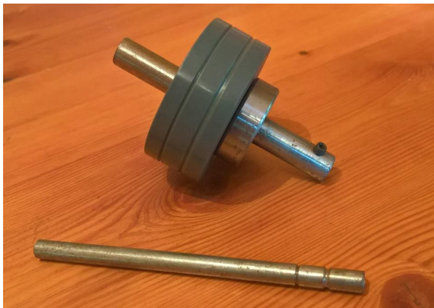
Figure 5.1.3 1: Initial Belt Transmission for the Turboshaft
