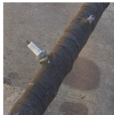
Figure 5.1.2 2: Flame Tube Fuel Inlet and Spark Plug
