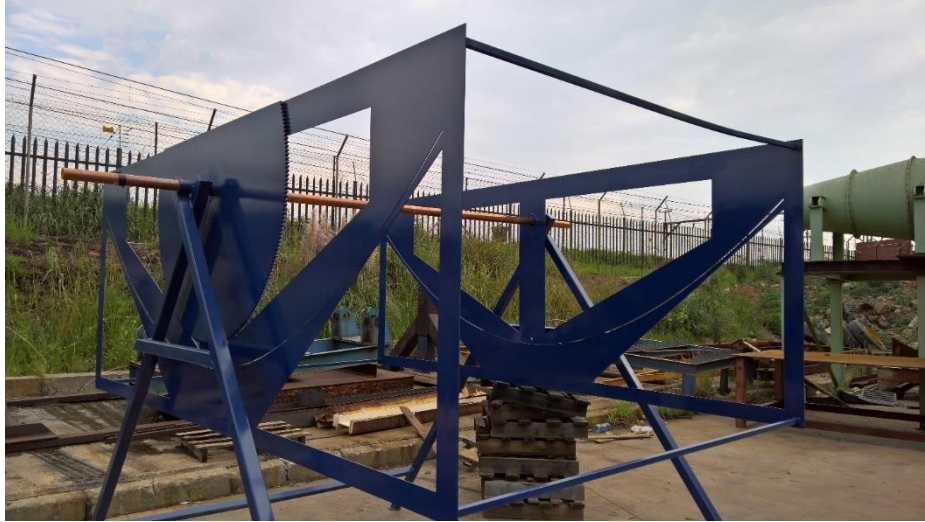
Figure 5.1.1 1: A Completed Frame and Mirror Brace Assembly
