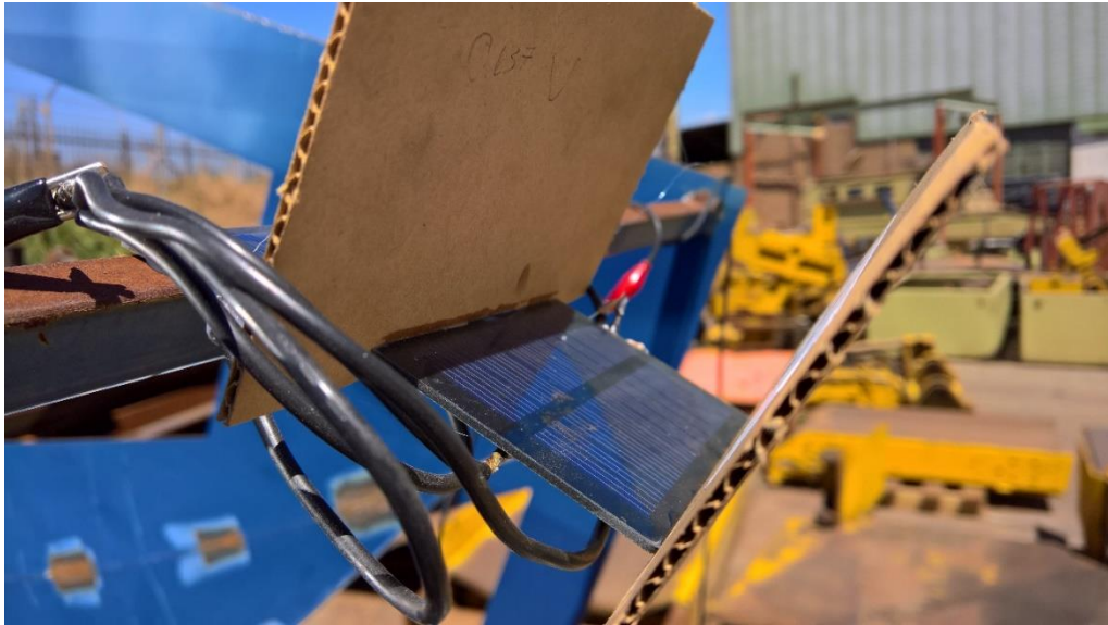
Figure 5.1.4 1: Solar Panel Shading Mechanism used by the Heliostat
