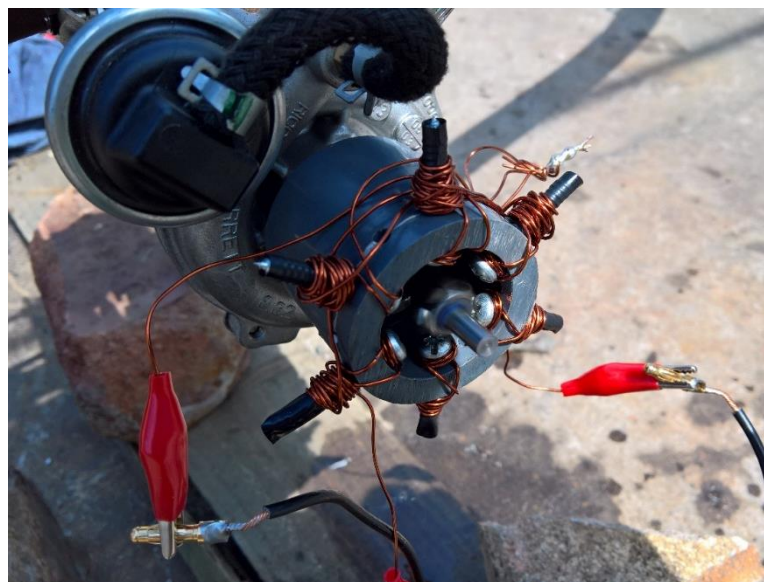
Figure 5.1.3 5: Gas Turbine Start-up using the Experimental In-runner BLDC Motor/Generator
