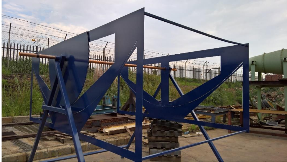
Figure D 2: A Completed Frame and Mirror Brace Assembly
