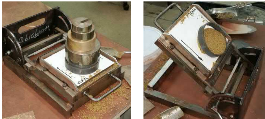
Figure 3-4 Inclined chute test of moist material on vinyl wall surface – slip at 38 degrees
