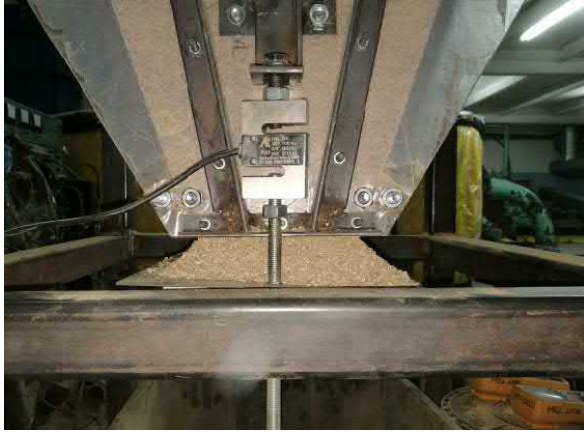
Figure B- 2 Sloped (dry) and near-vertical (moist) repose angles from dry and moist sand
