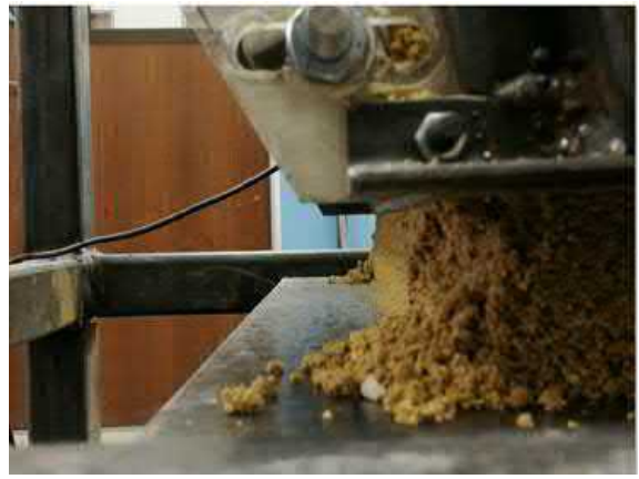
Figure B- 2 Sloped (dry) and near-vertical (moist) repose angles from dry and moist sand
