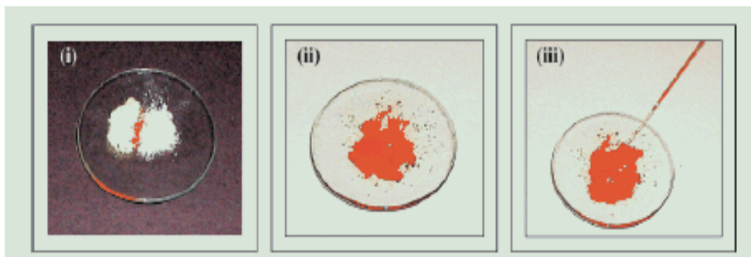
Figure 2.17: 4-aminotoluene and 2-hydroxy-3-methoxybenzaldehyde were ground separately. (i) Immediate orange liquid phase forms upon mixing at room temperature. (ii) Mixing with glass rod after 2 minutes, the entire mass is a homogenous liquid. (iii) Solid, orange azomethine product crystallizes from the liquid as the reaction proceeds and the entire mass is a wet crystalline solid in less than 10 minutes.
