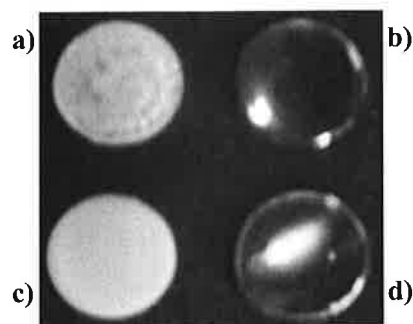
Figure 3.2. Digital images of the a) MTX-PLLA-PVA; b) PLLA-PVA; c) MTX-TEA-PLLA-PVA and d) TEA-PLLA-PVA biopolymeric membranes, where MTX=methotrexate; TEA=triethanolamine; PLLA=poly(L-lactic acid) and PVA=poly(vinyl alcohol).
