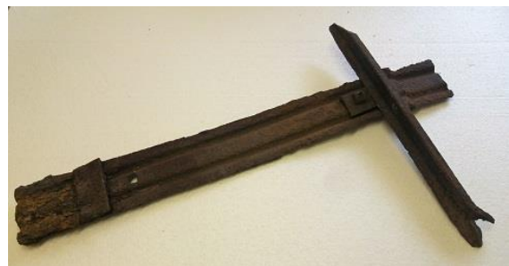
No 1025 Steel rail sleeper complete with bolted cleats shown with length of mine rail fitting perfectly
