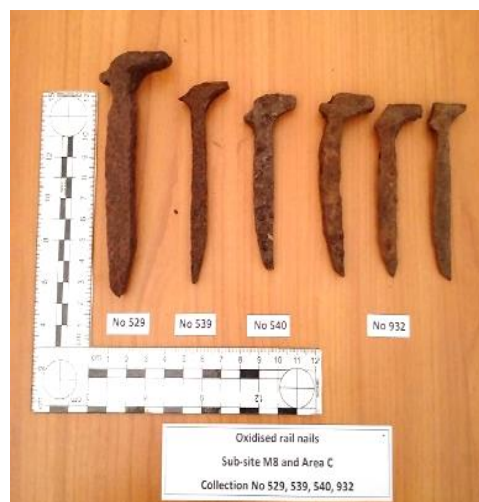
Hand forged rail nails c 1920s
