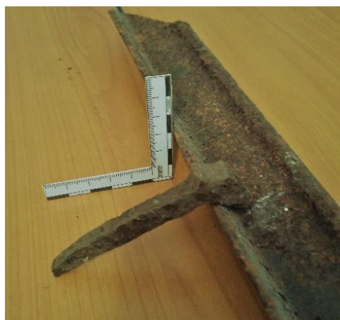
Figure 111. Argent rail nail fitting on the foot of a mine rail.
