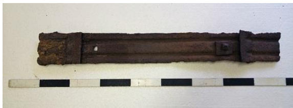
No 1025 Steel rail sleeper complete with bolted cleats shown with length of mine rail fitting perfectly
