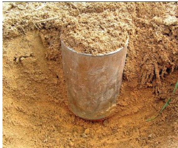
Figure 3.4: Steel ring (core) (Brown & Wherrett, 2018)
