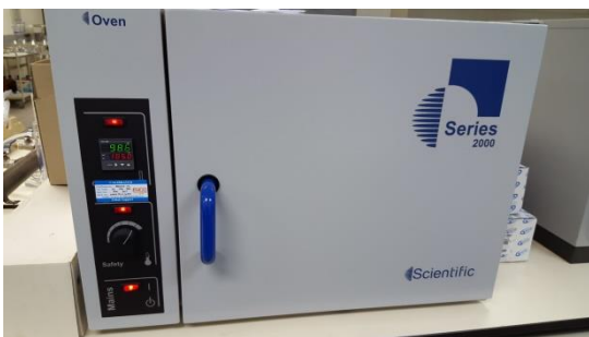
Figure 3.9: Oven set at 105 °C.
