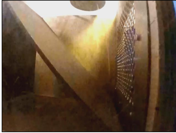
Figure 29: Close-up of physical experimental setup with mild steel deflector plate.
