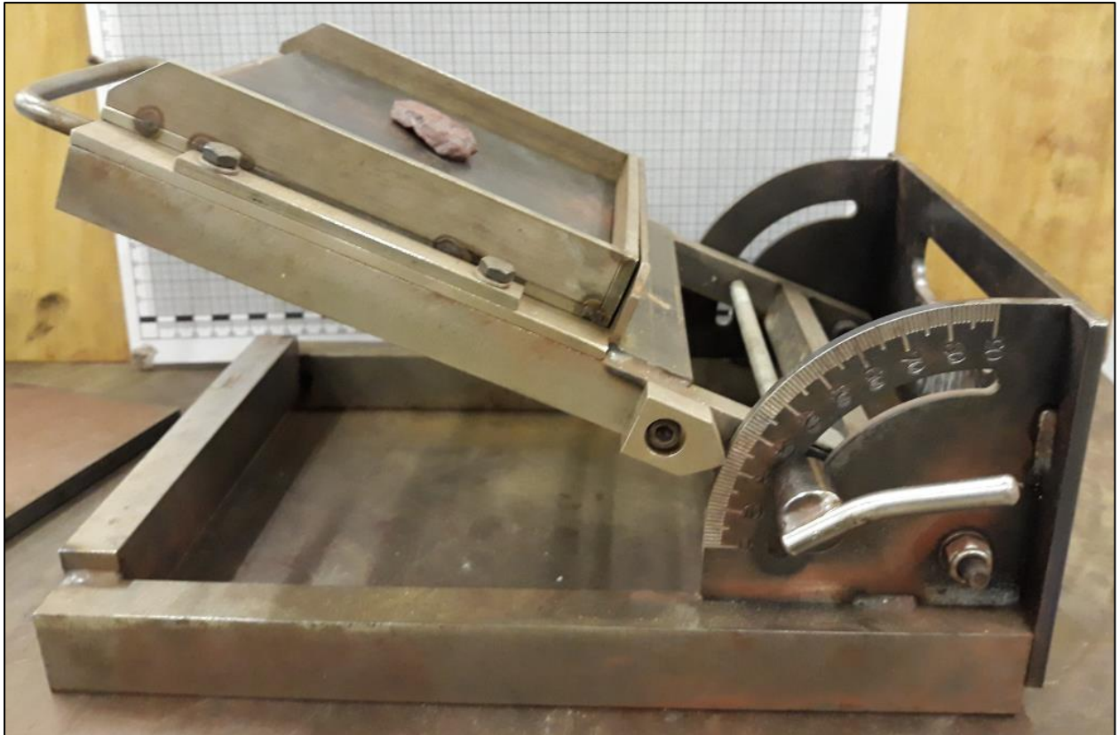
Figure 36: Position of the particle while plane is being inclined (current angle of 21°).
