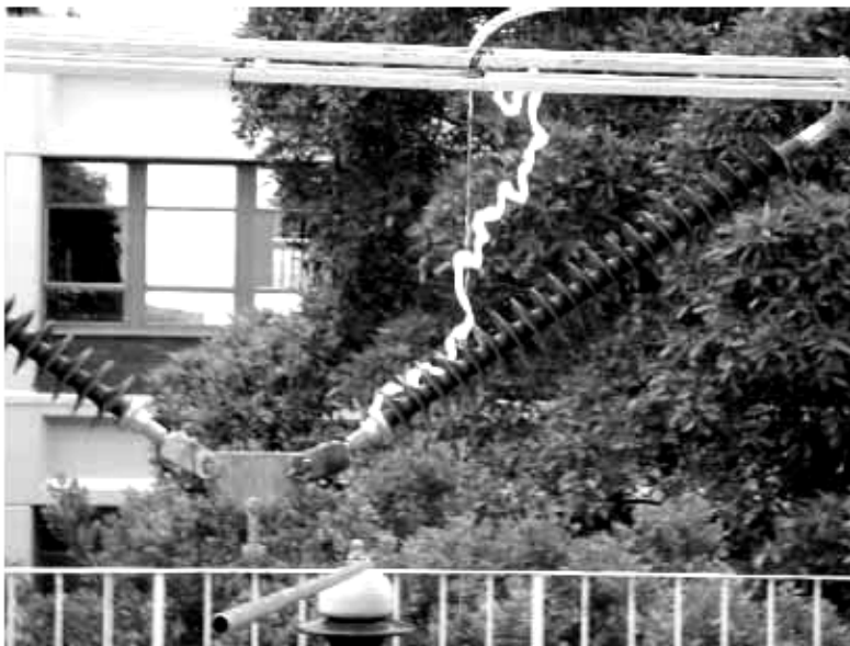
Figure 3 Bird streamer simulations performed on outdoor insulation system (Vosloo H. F., 2004).
