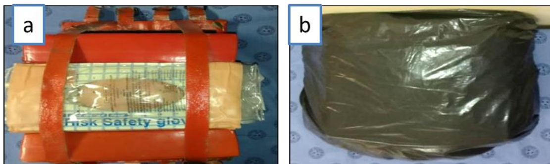
Figure 3: a) unit placed between head blocks, b) USCIT placed in black refuse bag
