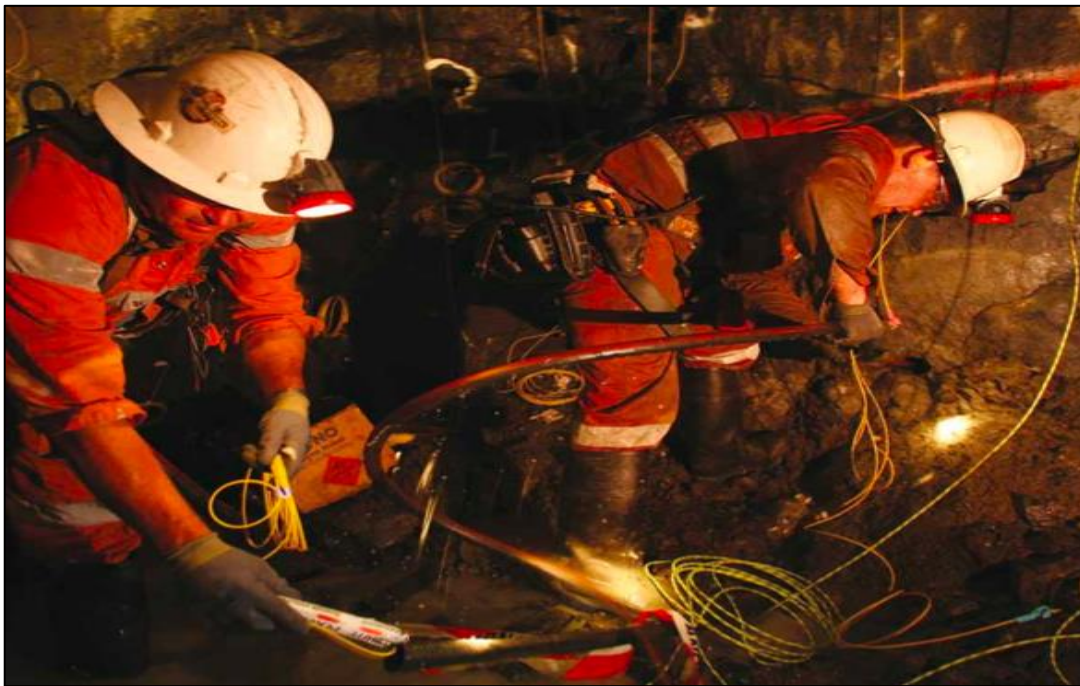
Figure 24: Charging an Underground Stope with Cartridge Explosives (Dyno Nobel, 2010)
