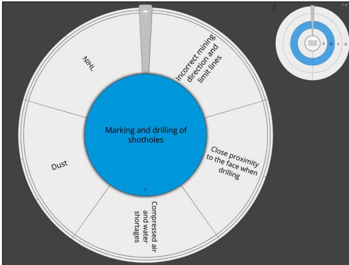
Figure 46: Challenges During Marking and Drilling of Shotholes
