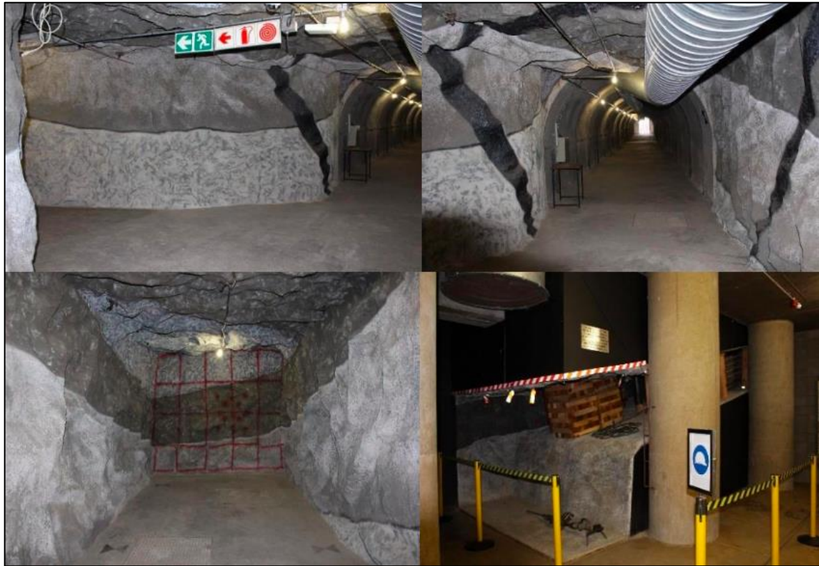
Figure 74: Crosscut, Development End and a Stope (Javaid, 2018)
