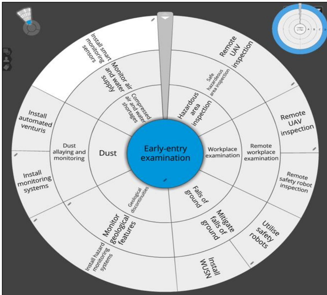
Figure 42: Digital Technology for the Early-entry Examination Phase
