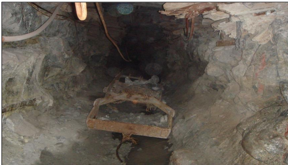
Figure 25: Scraper Winch Scoop Pulling Ore (Phakathi, 2017)
