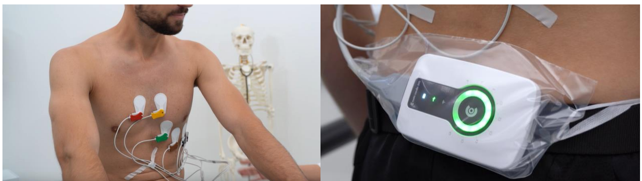
Figure 3.22 Customed ECG system
