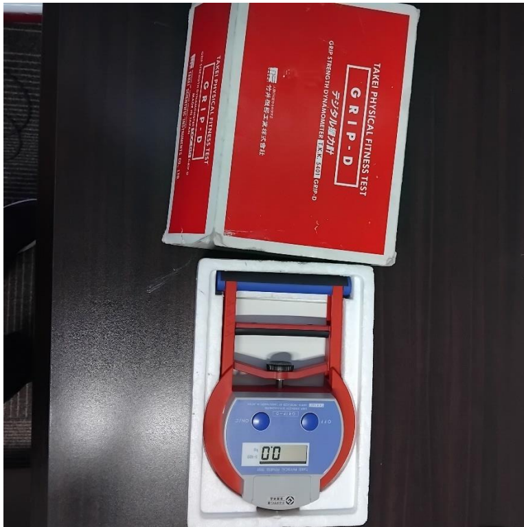
Figure 3.21 Takei™ grip-D handgrip dynamometer
