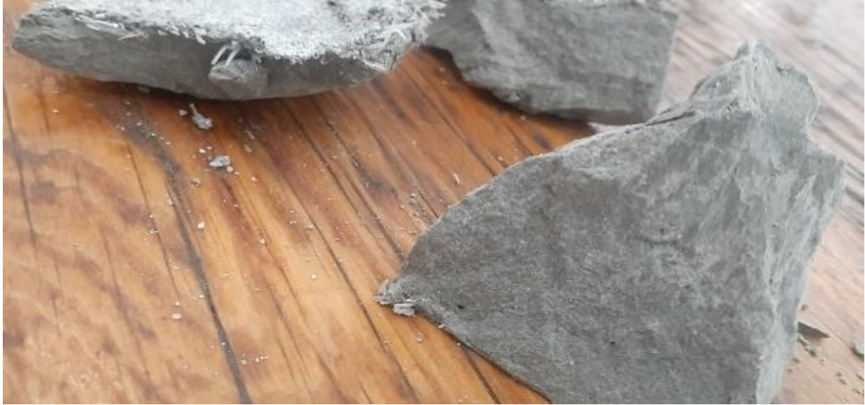
Figure 8: Set Oil Well Cement Specimen Incorporated with Short PET Fibres After a Destructive Compressive Strength Test.
