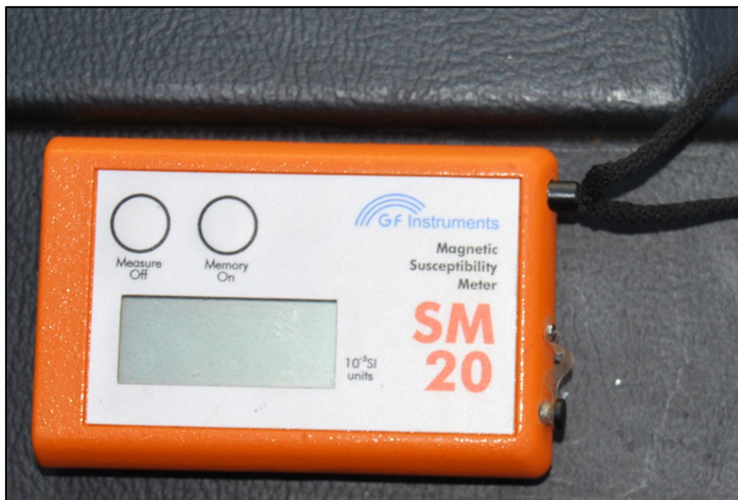
Figure 7.6 A photograph of the handheld SM 20 magnetic susceptibility meter.
