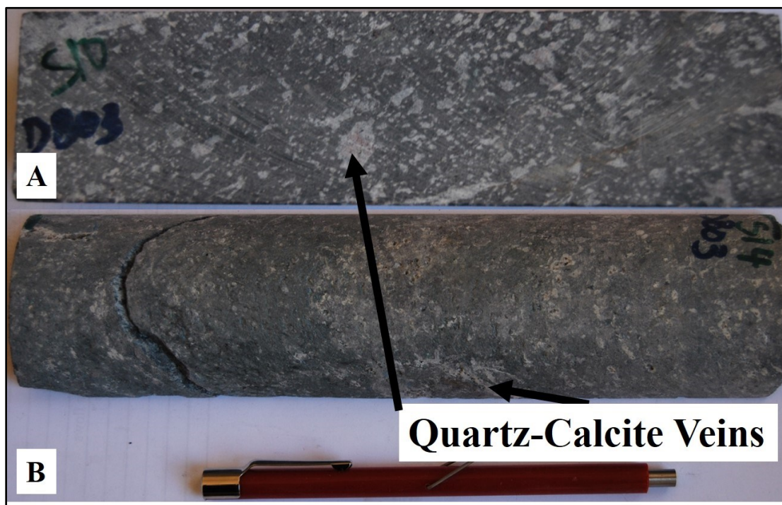
Figure 3.8 Photographs of the tuff. A) Half drill core of the tuff with frequent quartz-calcite veins. DBDD0003: 39.20 m – 39.40 m – DB3S10. B) Half drill core of the tuff with quartz-calcite veins and numerous calcite vugs. DBDD0003: 67.40 m – 67.60 m – DB3S14. Magnetic pen for scale.
