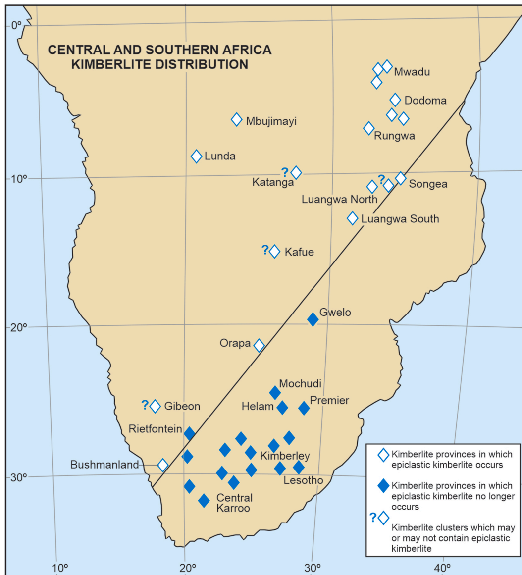
Fig. 18. Distribution of kimberlites in central and southern Africa with known and possible preserved crater-lake sedimentary sequences, which are separated by the NE-SW diagonal line from eroded pipes lacking crater-fill sedimentary cappings. (Adapted from Hawthorne, 1975).
