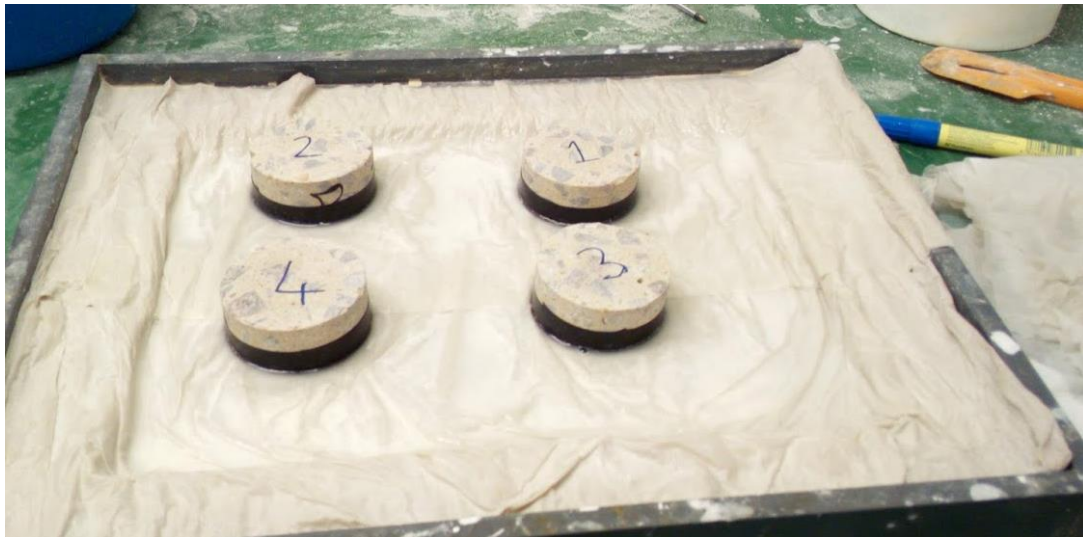
Figure 3-26 - Water sorptivity test set up
