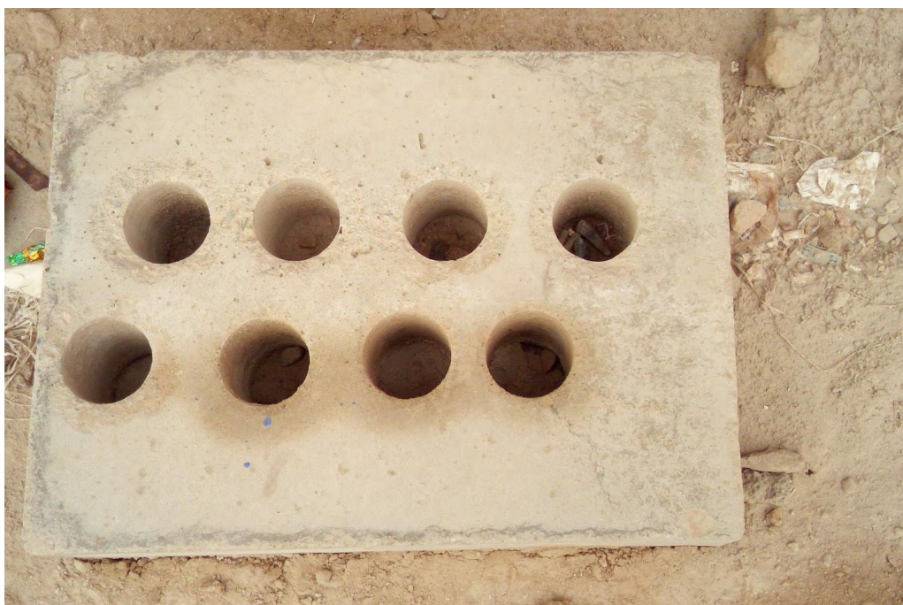
Figure 3-24 - Cores removed from sample panels
