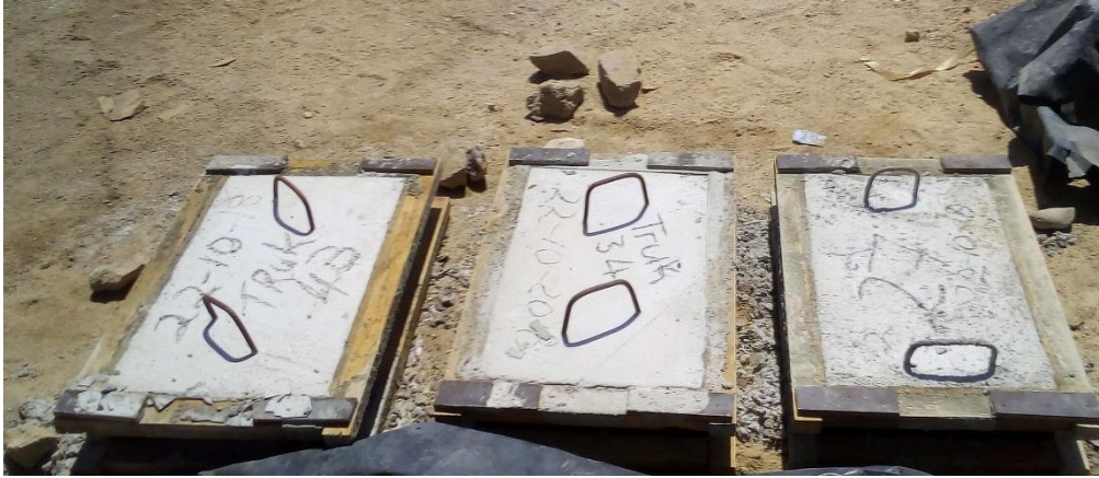
Figure 3-22 - Durability test panels representing bridge deck
