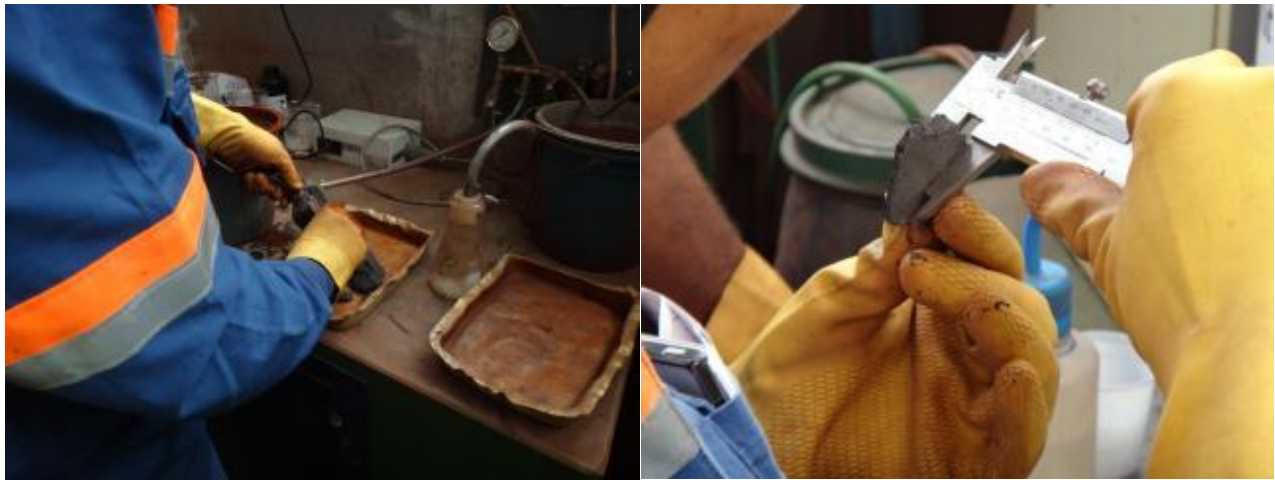
Figure 3.5: Cake discharge and measuring of cake thickness.
