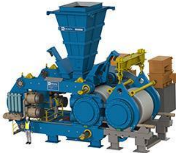
Figure 2.7: Schematic of a typical HPGR (FLSmidth & Co., 2014).
