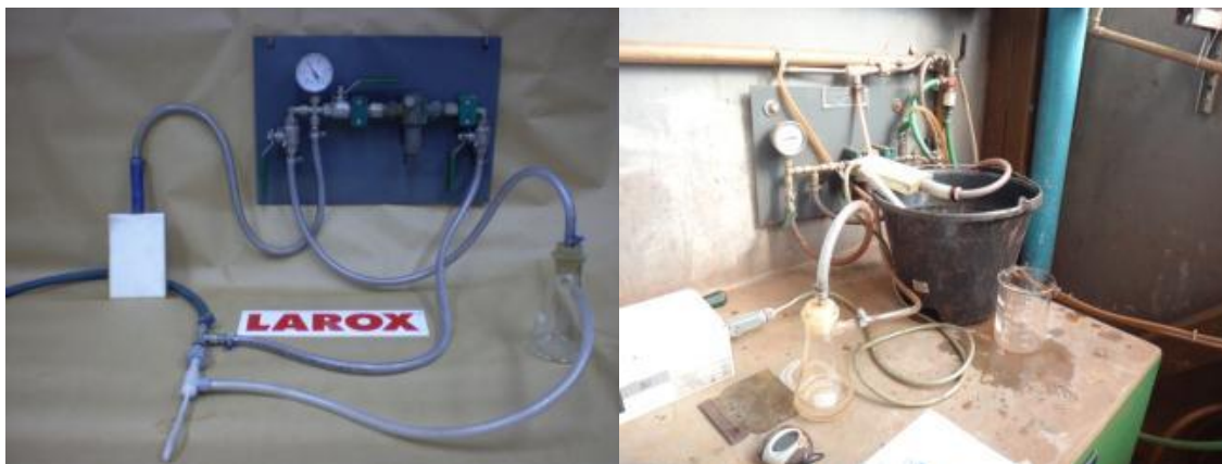
Figure 3.1: Larox ceramic leaf tester (left) and actual leaf testing unit at the operation's pilot facility (right).
