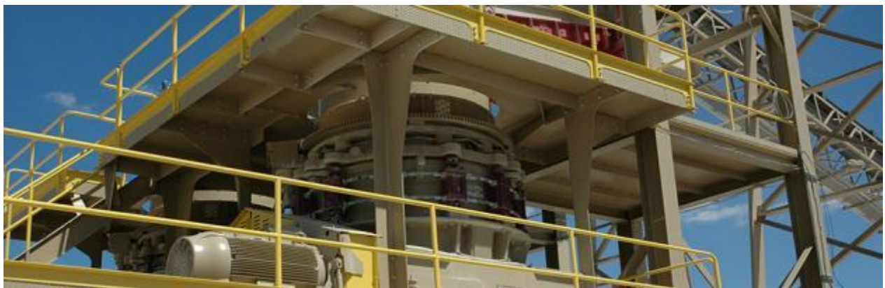
Figure 2.6: Cone crusher (Astec Industries Inc, 2014).
