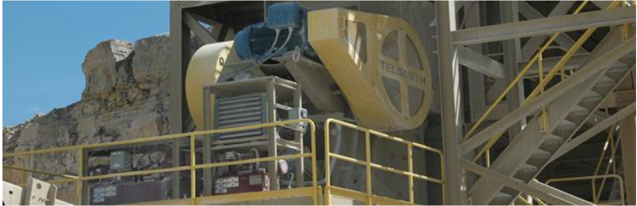
Figure 2.5: Jaw crusher (Astec Industries Inc, 2014).
