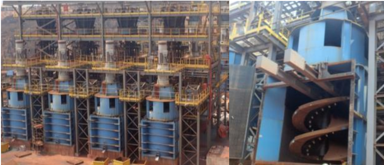
Figure 2.14: Verti mills at the Minas-Rio operation.
