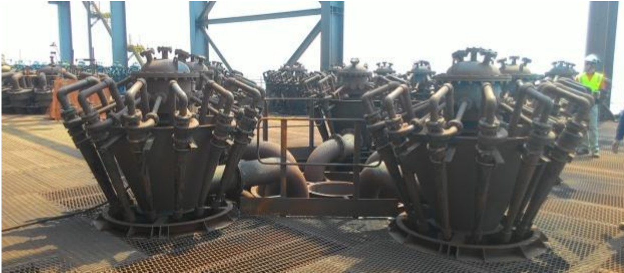
Figure 2.11: Hydrocyclone clusters located at the Minas-Rio operation.
