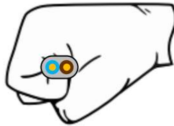
Figure 9 – Hand grasping a flat power cable, with cable in the cross-sectional view. Blue and brown circles indicates insulation around the neutral and live wire, respectively. Human fist outline adapted from Wikimedia Commons [52].
