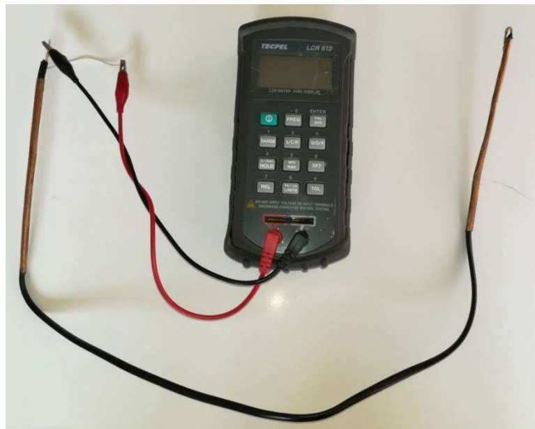
Figure 30 – Hand-to-hand Impedance measurement setup. A Type P3 (2 × 0.75mm) cable was wrapped with copper tape on its end. The brown wire was connected to the copper plate on the left to the red node of the LCR meter. The black node was connected to the right copper plate with a jumper wire.
