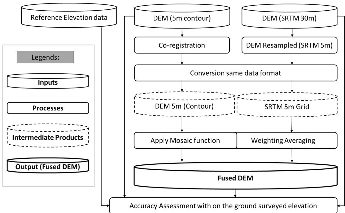
Figure 3.2 Workflow of the DEMs fusion algorithm: algorithm adapted after Karkee et al (2008).
