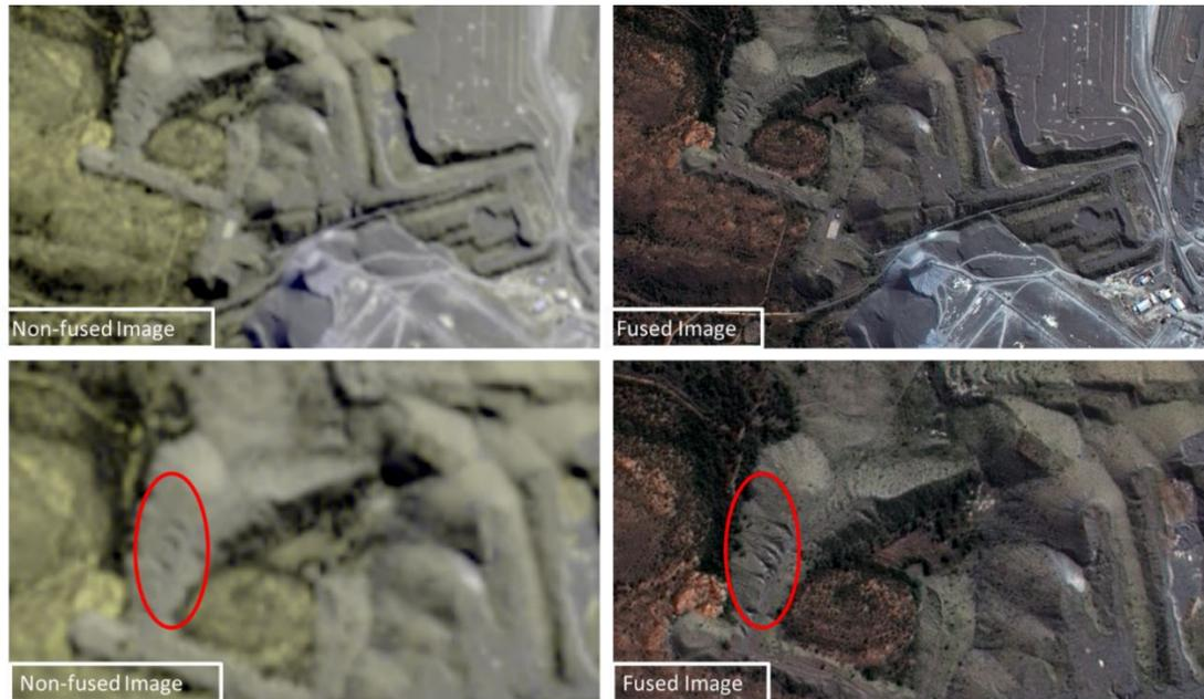
Figure 3.4 Pan-sharpened SPOT-6 (1.5 m) image (Right panels: Non-fused) with an improved resolution image compared with 6m–multispectral image (Left-hand panels) for better interpretation of tailings erosion highlighted in red oval shapes.
